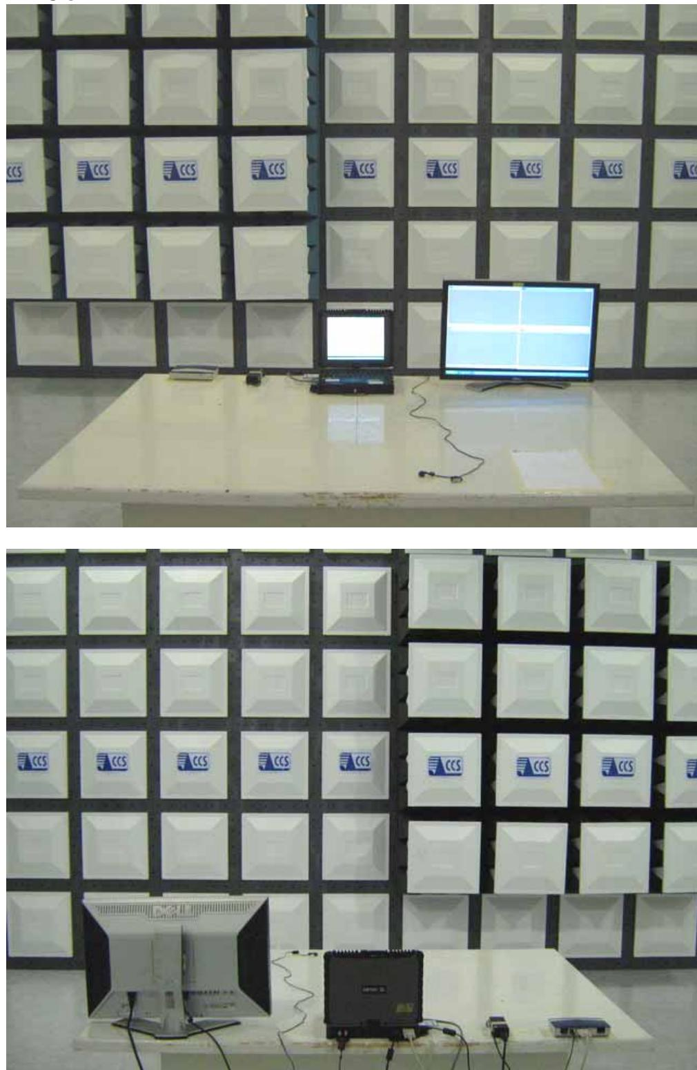
**POWERLINE CONDUCTED EMISSIONS MEASUREMENT SETUP****EMC-1**
