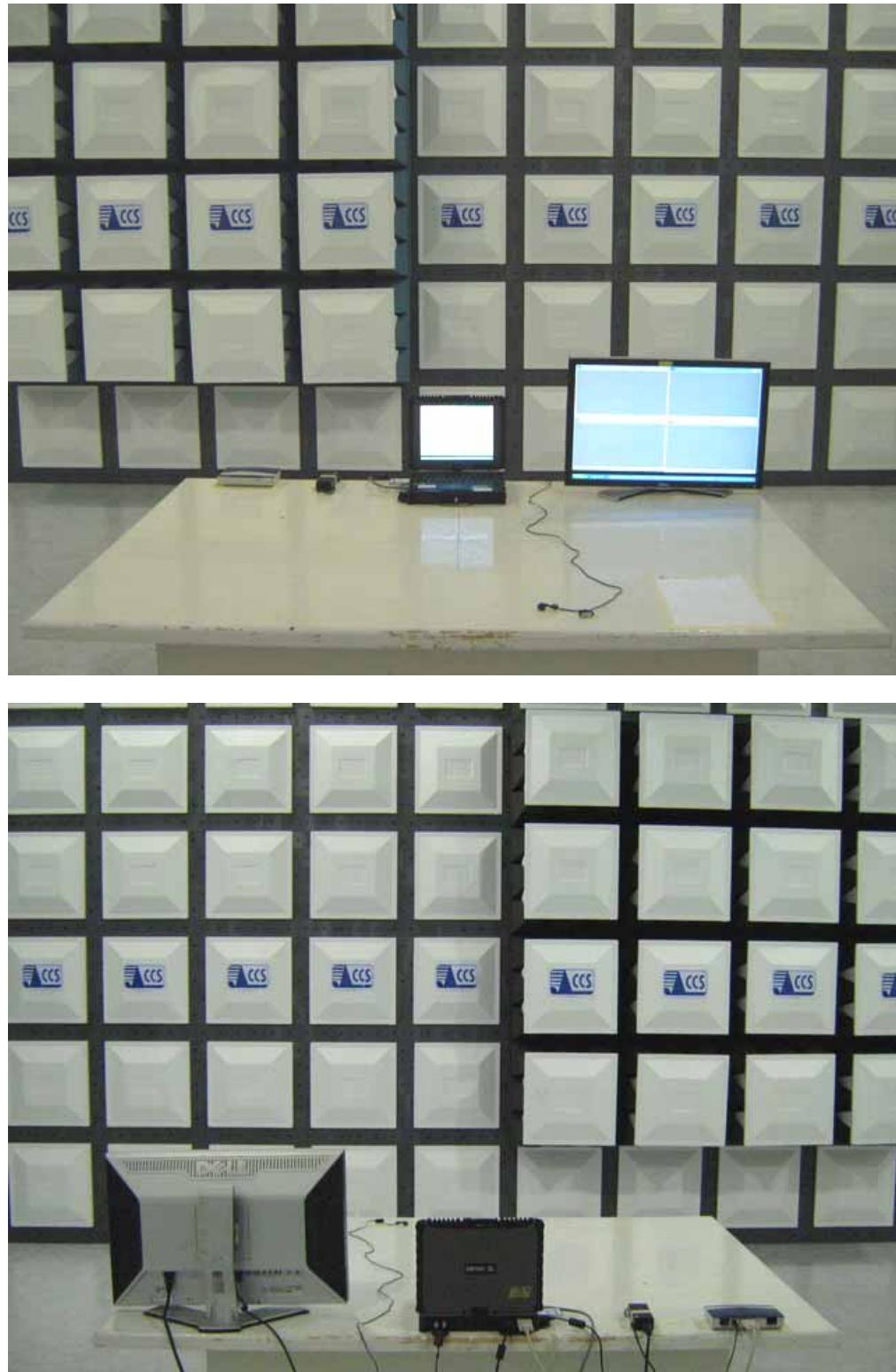
**POWERLINE CONDUCTED EMISSIONS MEASUREMENT SETUP****EMC-1**
