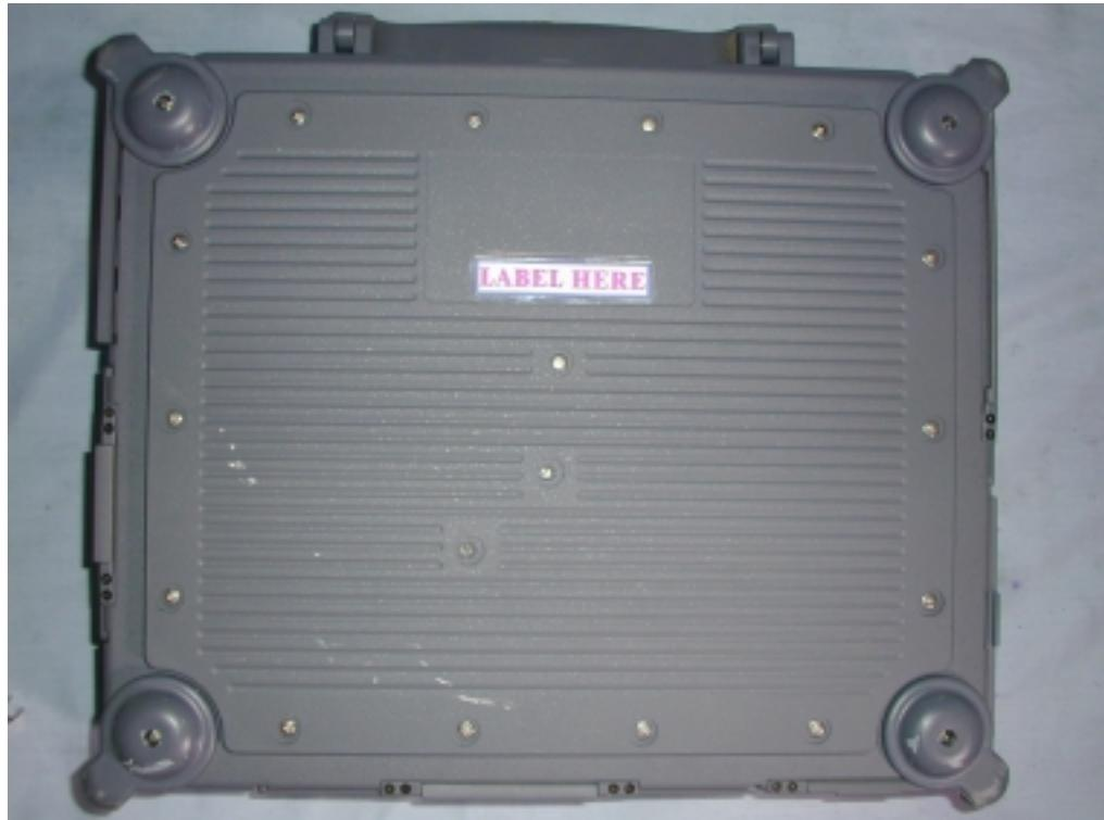
The FCC ID Label will be placed on the equipment as shown in the photograph.
