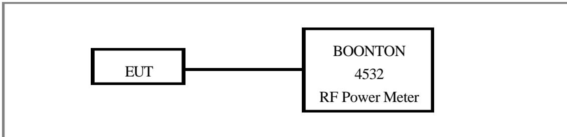
1. The output of the transmitter is connected to the BOONTON RF Power Meter.
