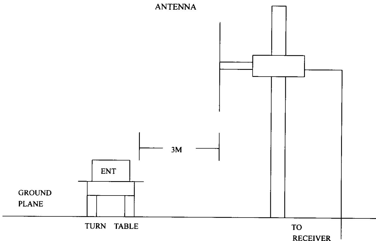
**6 . 3 RADIATED TEST SET-UP**
