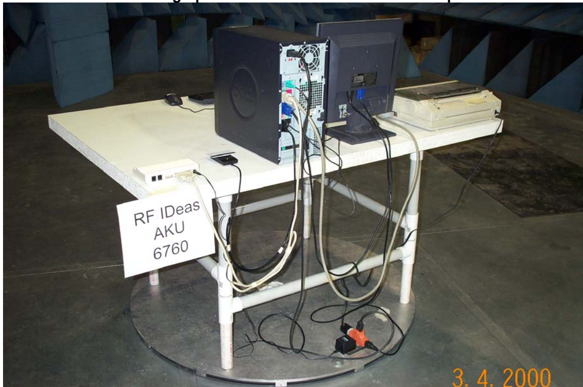
Photograph of Radiated Emissions Test Setup
