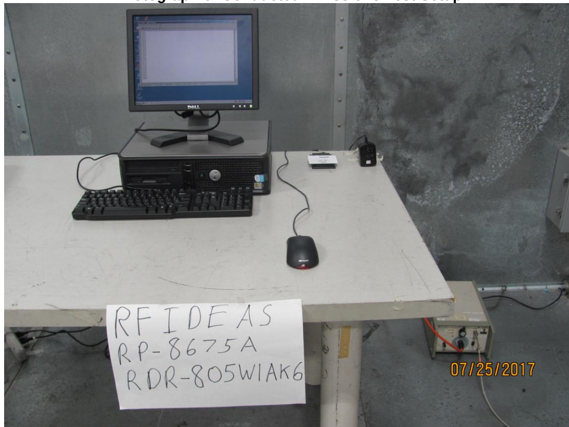
Photograph of Conducted Emissions Test Setup
