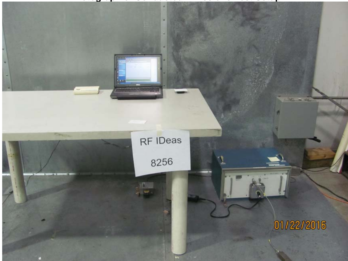
Photograph of Conducted Emissions Test Setup
