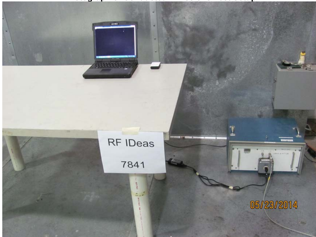
Photograph of Conducted Emissions Test Setup
