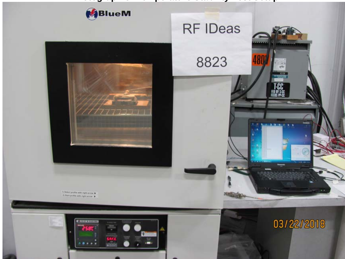
Photograph of Temperature Stability Test Setup
