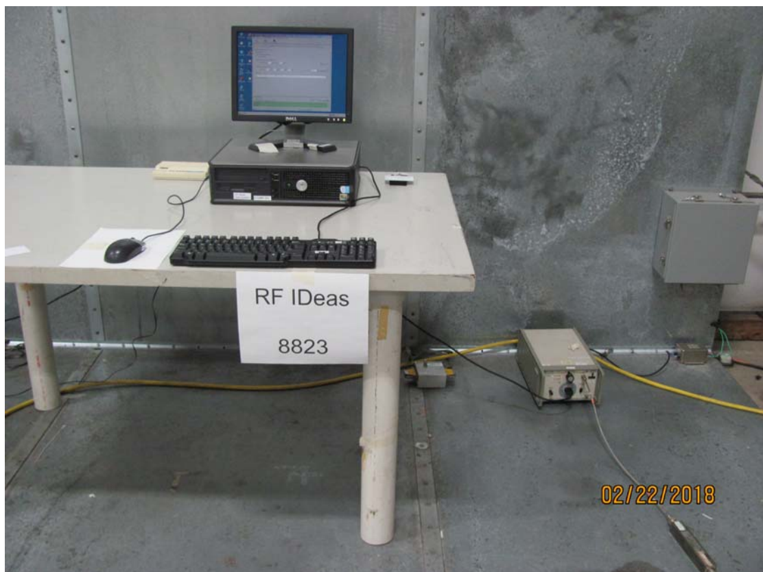
Photograph of Conducted Emissions Test Setup
