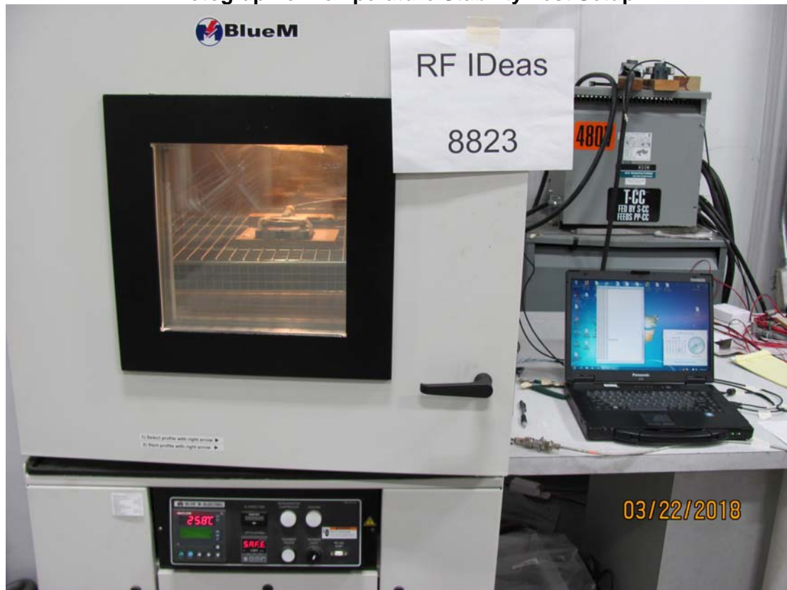
Photograph of Temperature Stability Test Setup
