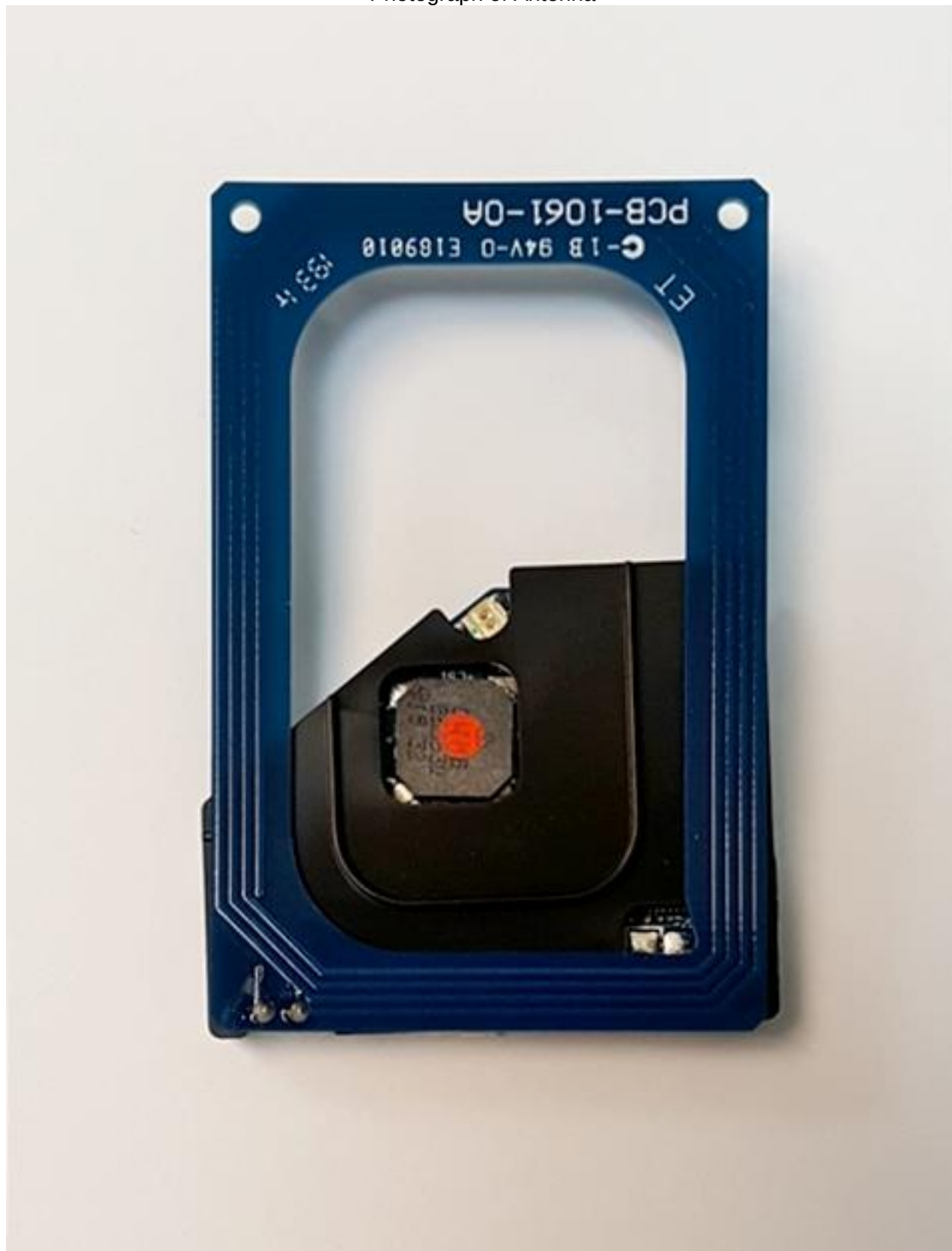
Photograph of Antenna
