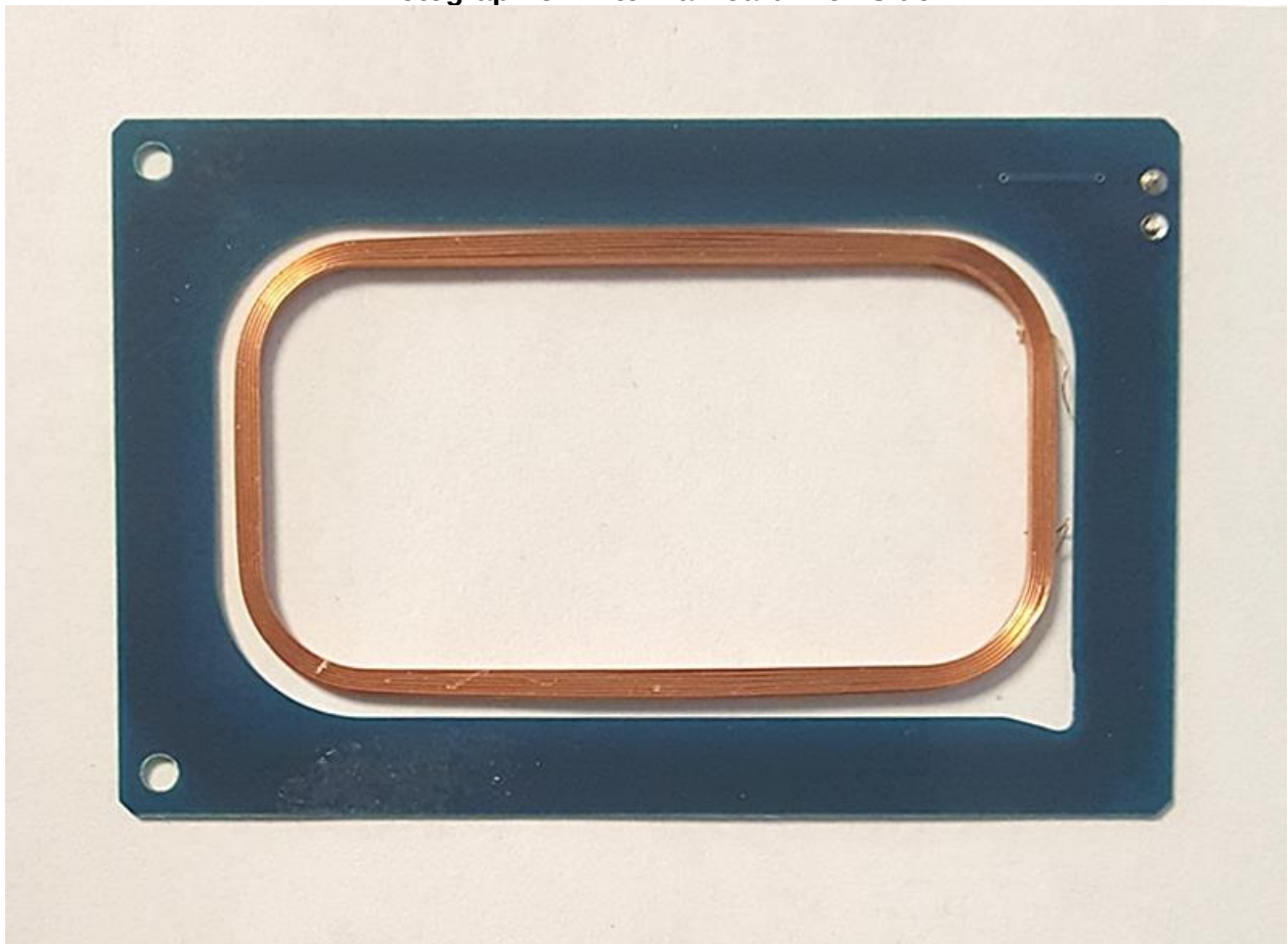
Photograph of Antenna Board: Foil Side
