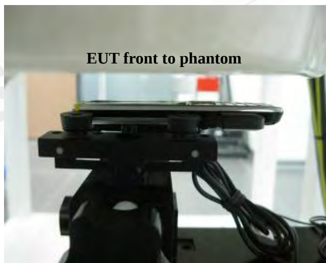
Fig.9 Body worn- EUT front to flat phantom and distance between flat phantom and mobile phone is 1.5 cm with headset
