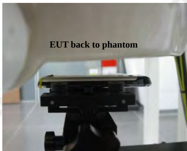
Fig.8 Body worn- EUT back to flat phantom and distance between flat phantom and mobile phone is 1.5 cm
