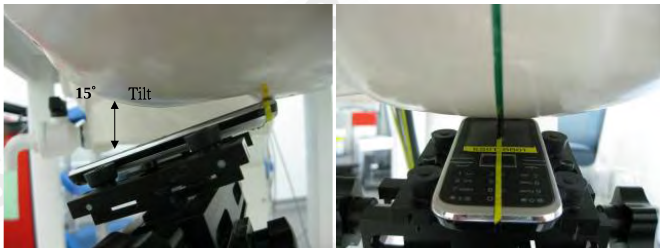
Fig.6 Left Head at Ear-Tilt Position(15°)
