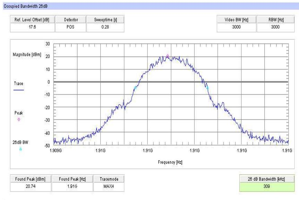
**Channel 512 (EDGE)****99% (-20 dB) Occupied Bandwidth**
