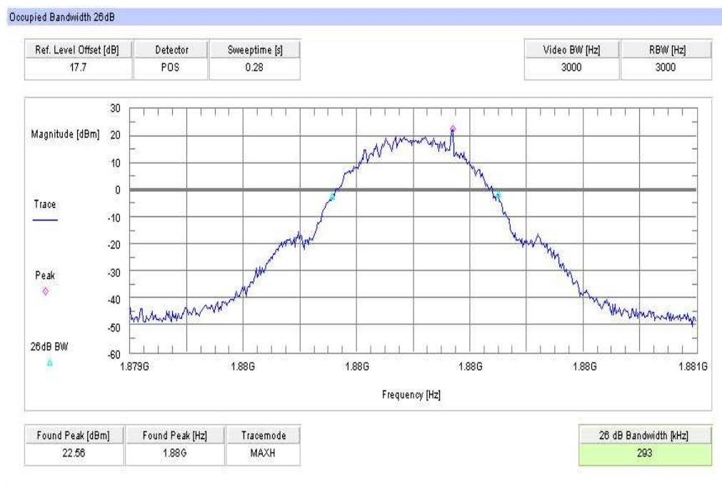
**Channel 810****99% (-20 dB) Occupied Bandwidth**
