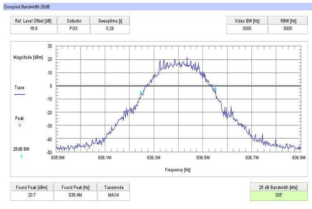
**Channel 251 (EDGE)****99% (-20 dB) Occupied Bandwidth**
