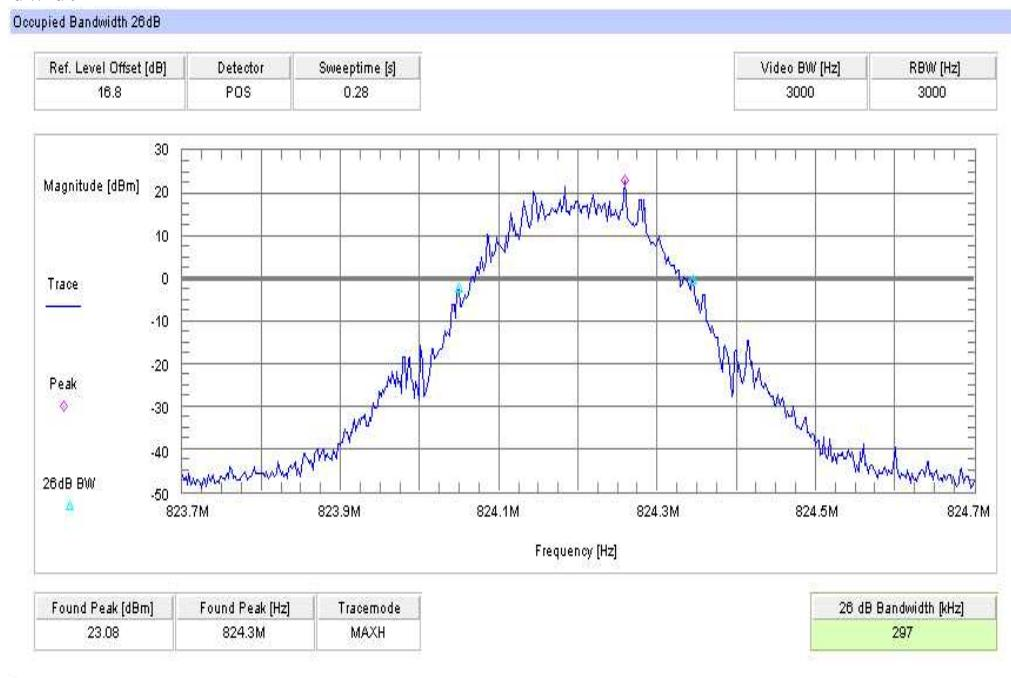
**Channel 189 (EDGE)****99% (-20 dB) Occupied Bandwidth**
