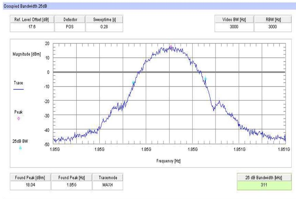
**Channel 661 (EDGE)****99% (-20 dB) Occupied Bandwidth**
