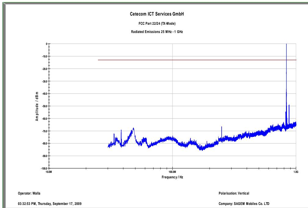
$f < 1 \text{ GHz}$  : RBW/VBW: 100 kHz $f \geq 1 \text{ GHz}$  : RBW / VBW 1 MHz**Channel 189 (30 MHz - 1 GHz) – Antenna Horizontal**
