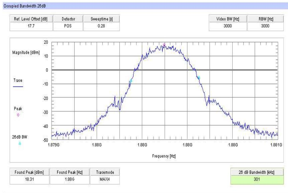
**Channel 810 (EDGE)****99% (-20 dB) Occupied Bandwidth**
