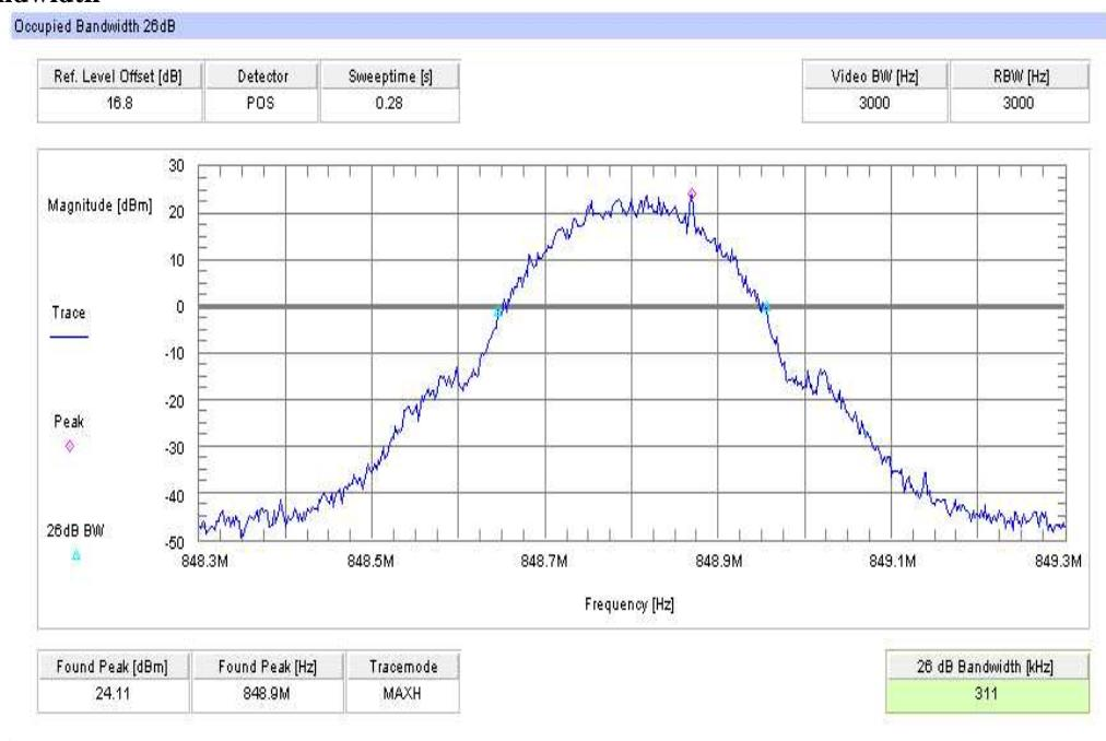
**Channel 128 (EDGE)****99% (-20 dB) Occupied Bandwidth**
