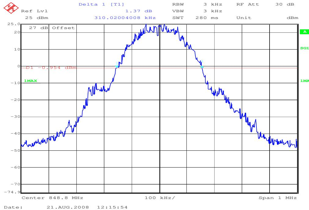
**Channel 128 (EDGE)****99% (-20 dB) Occupied Bandwidth**
