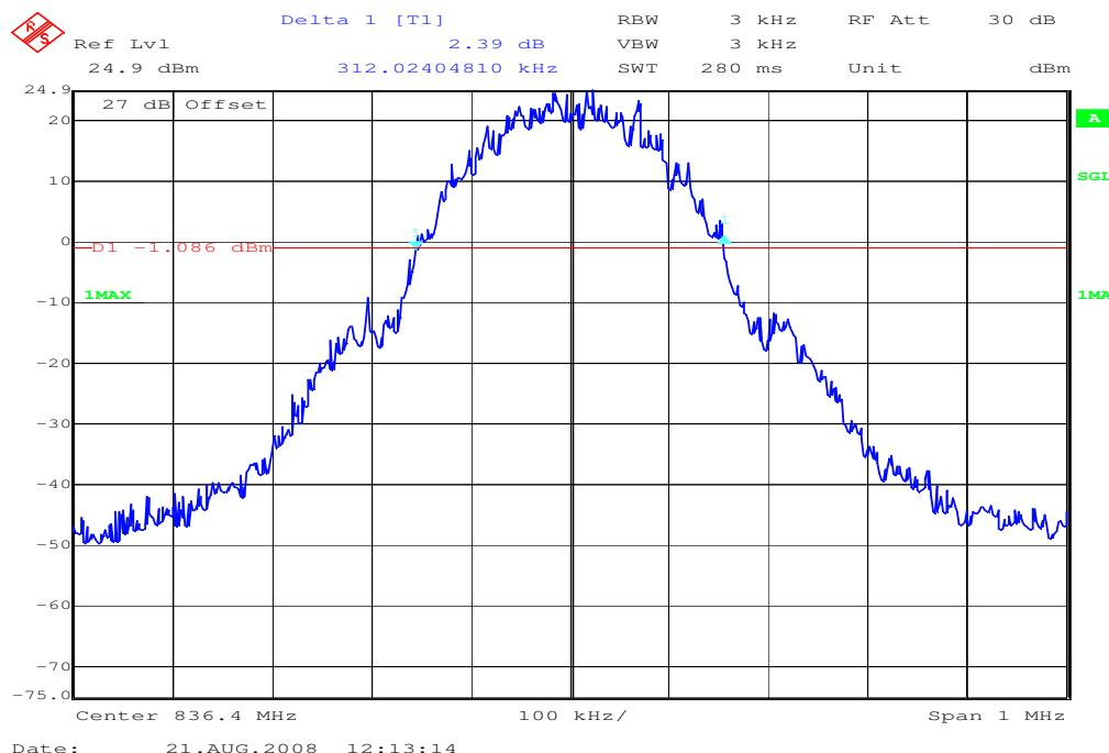
**Channel 251****99% (-20 dB) Occupied Bandwidth**
