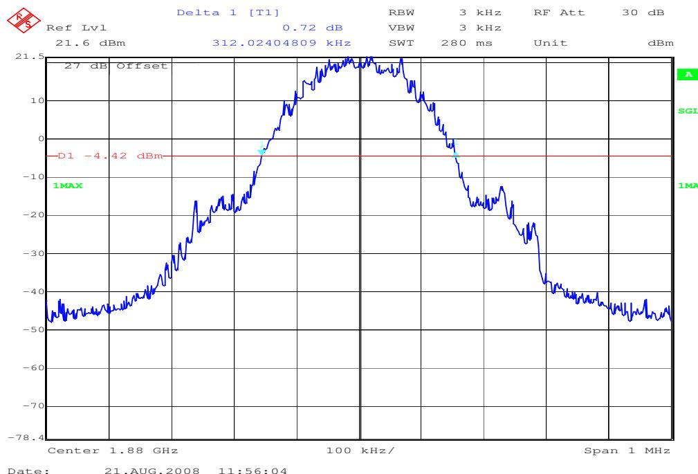
**Channel 810****99% (-20 dB) Occupied Bandwidth**
