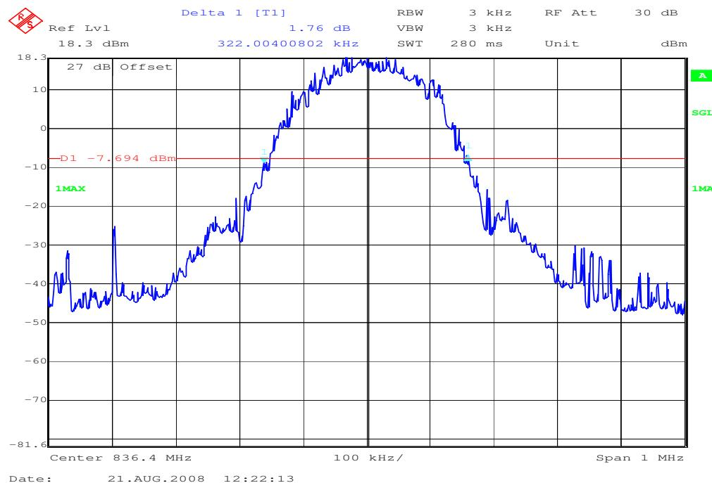
**Channel 251 (EDGE)****99% (-20 dB) Occupied Bandwidth**
