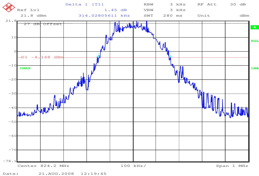
**Channel 189 (EDGE)****99% (-20 dB) Occupied Bandwidth**
