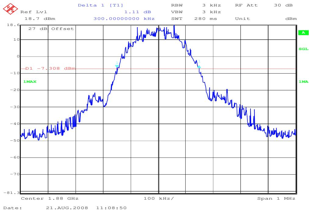
**Channel 810 (EDGE)****99% (-20 dB) Occupied Bandwidth**
