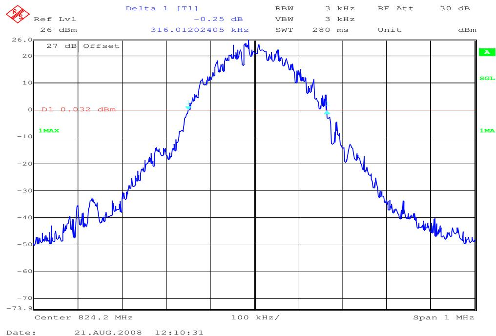
**Channel 189****99% (-20 dB) Occupied Bandwidth**
