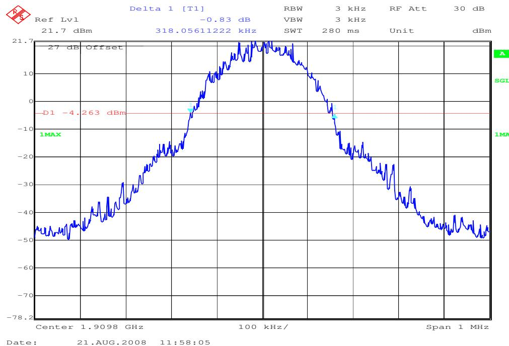
**Channel 512 (EDGE)****99% (-20 dB) Occupied Bandwidth**
