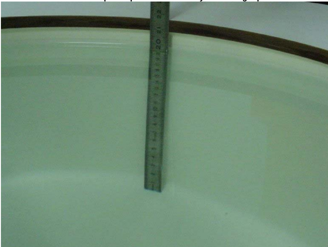
Photo 4: Liquid depth 1900 MHz body simulating liquid
