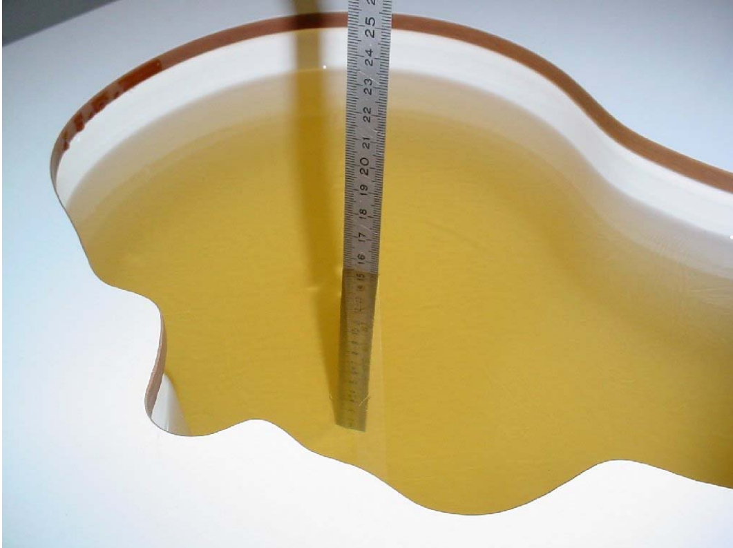
Photo 2: Liquid depth 850 MHz body simulating liquid
