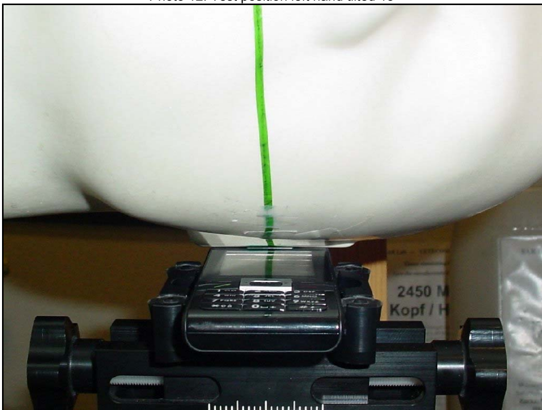
Photo 12: Test position left hand tilted 15°
