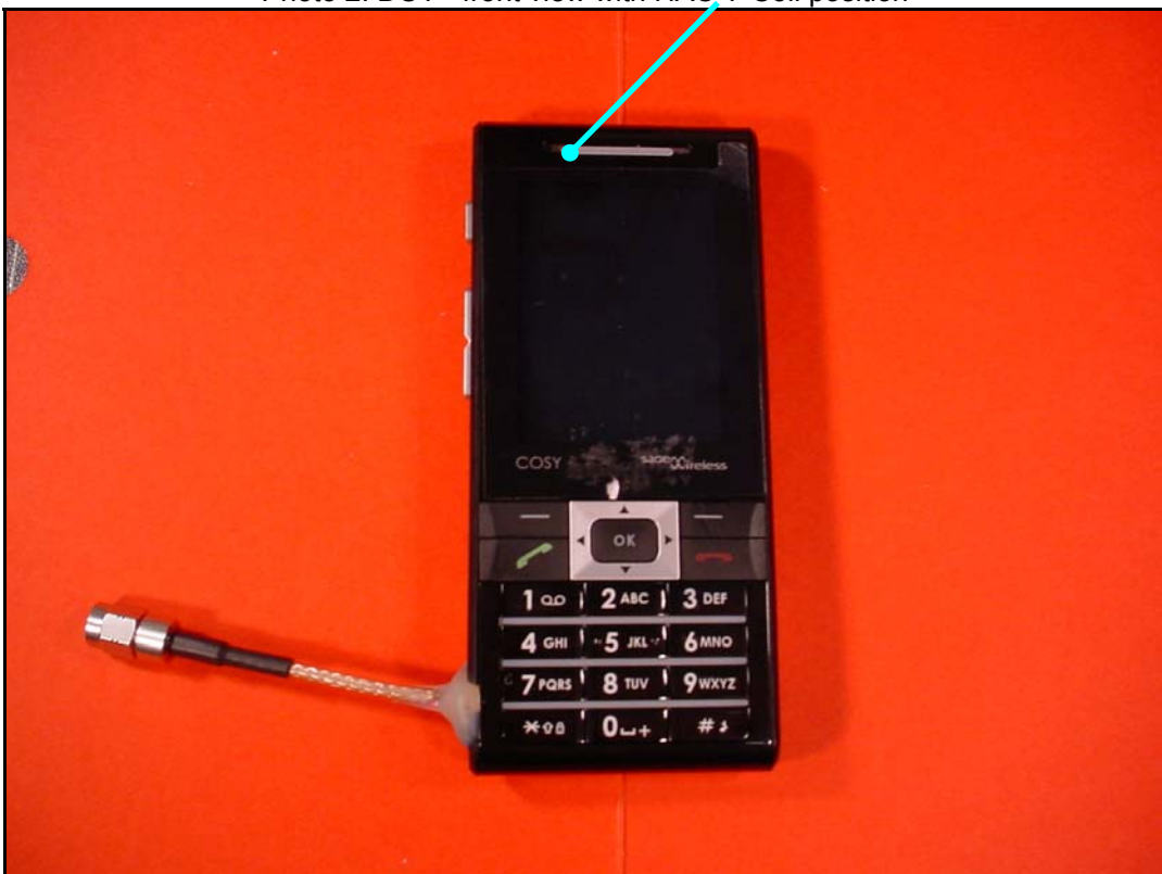
Photo 2: DUT - front view with HAC T-Coil position
