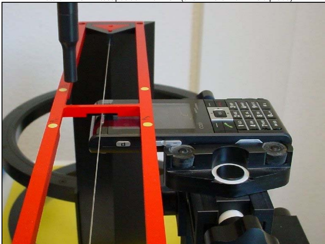
Photo 6: HAC RF test position with DUT (shown here with E-field probe)
