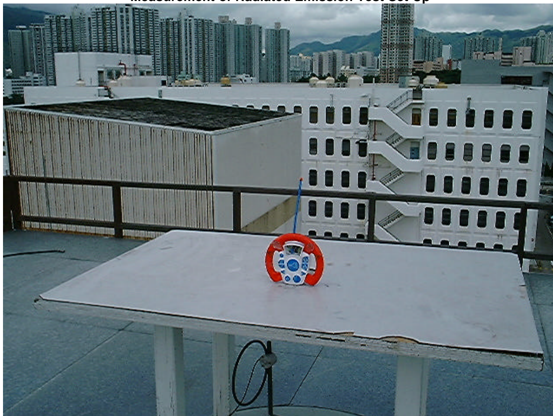
Measurement of Radiated Emission Test Set Up
