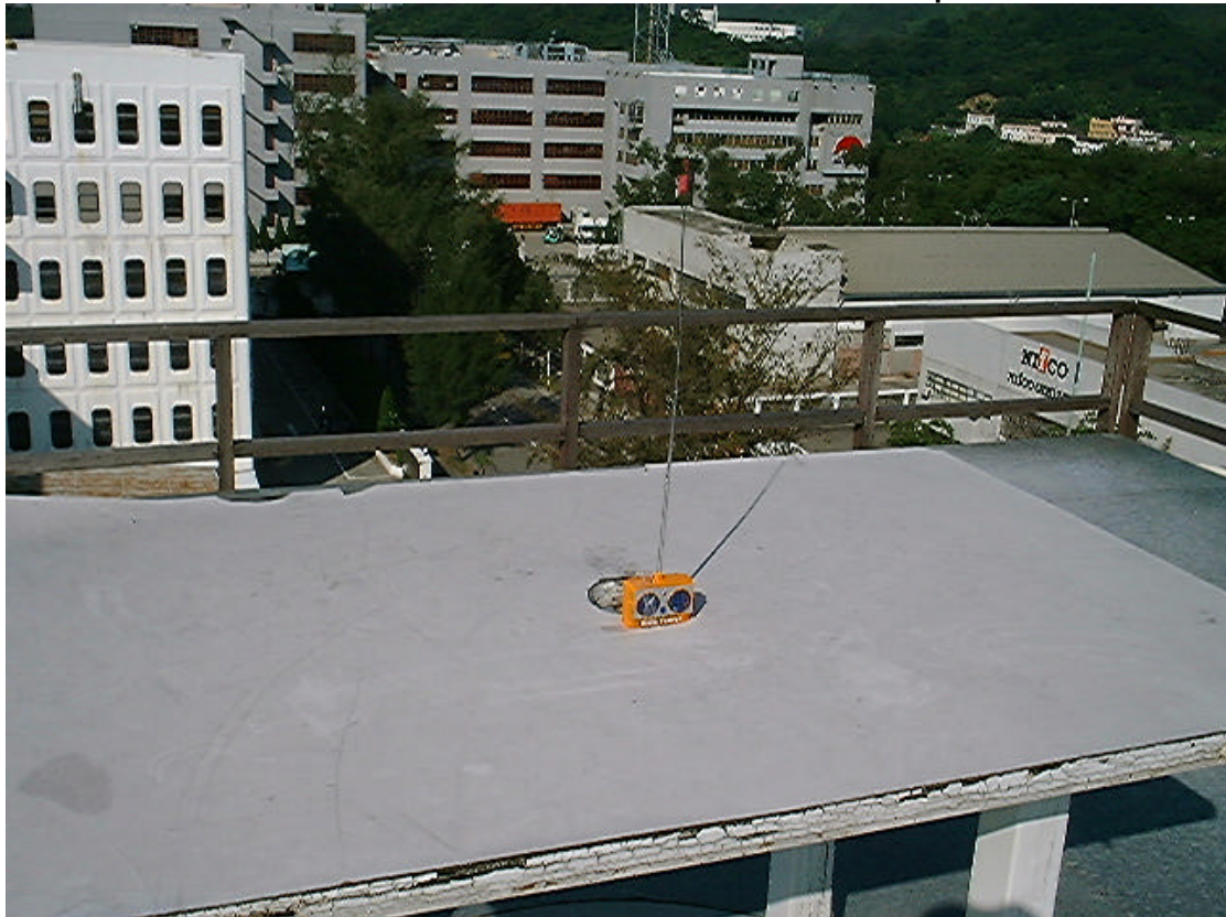
Measurement of Radiated Emission Test Set Up
