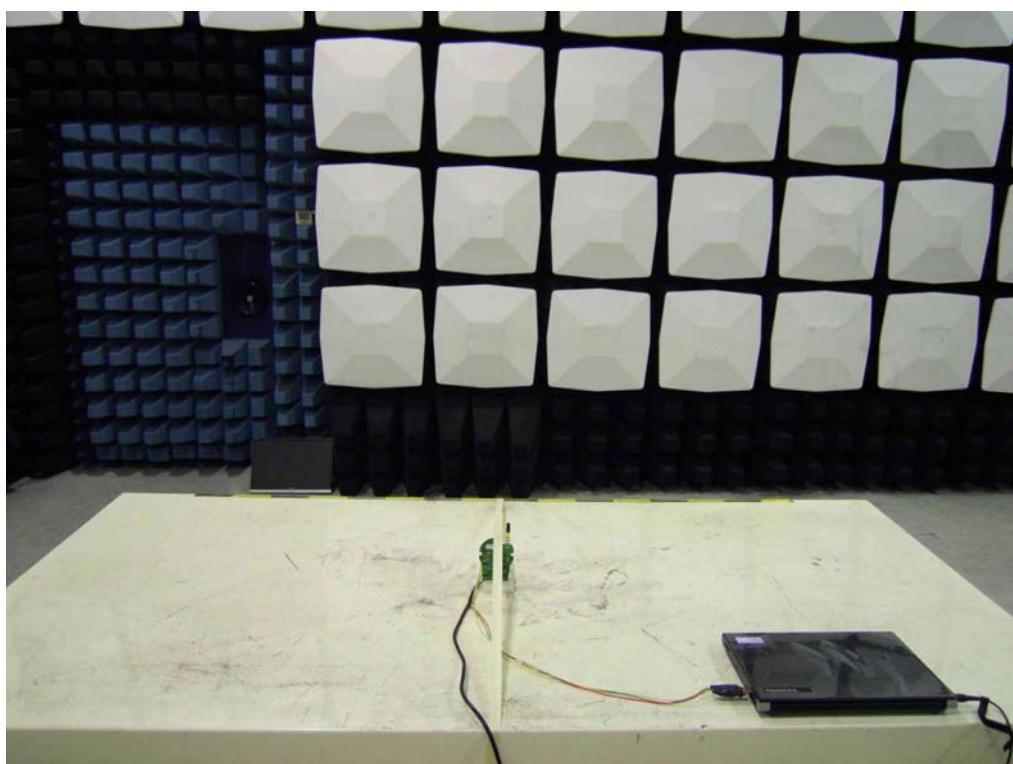
**ANTENNA PORT CONDUCTED RF MEASUREMENT SETUP**
