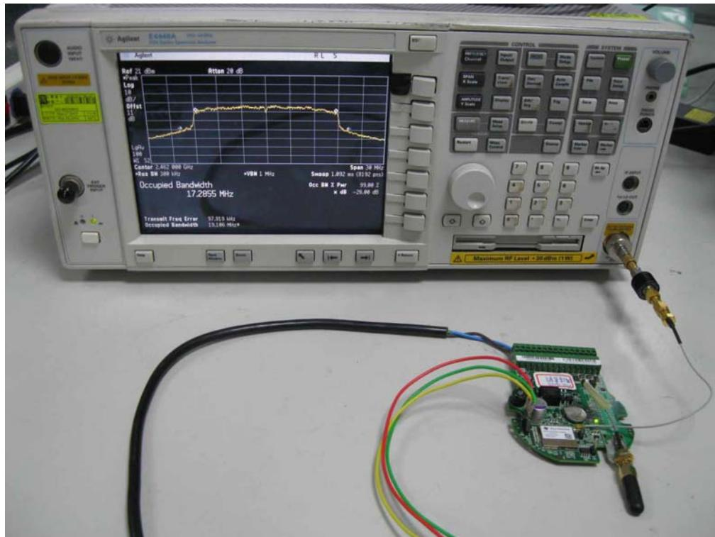
**CONDUCTED EMISSION SETUP**
