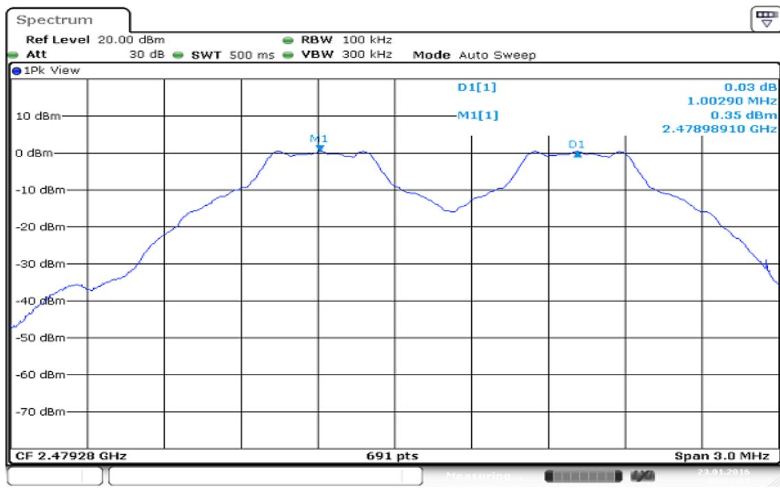
**For 8DPSK / DH5****Measurement of Channel Separation / (CH Low)**
