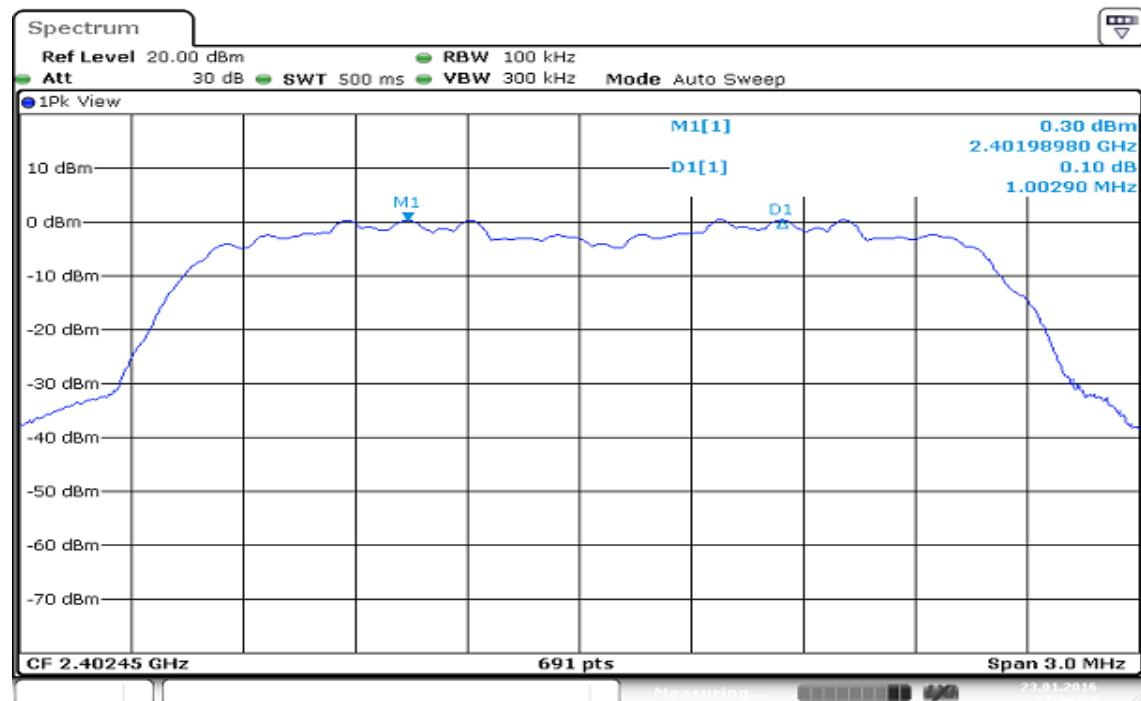
**Measurement of Channel Separation / (CH Mid)**
