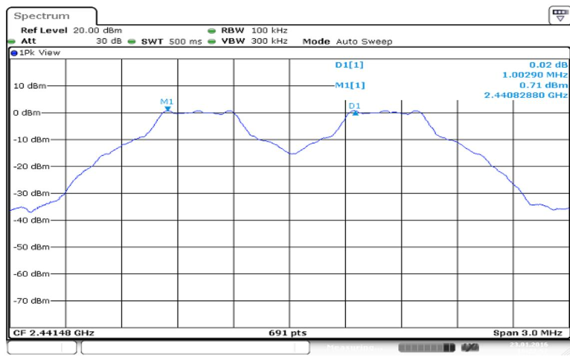
**Measurement of Channel Separation / (CH High)**
