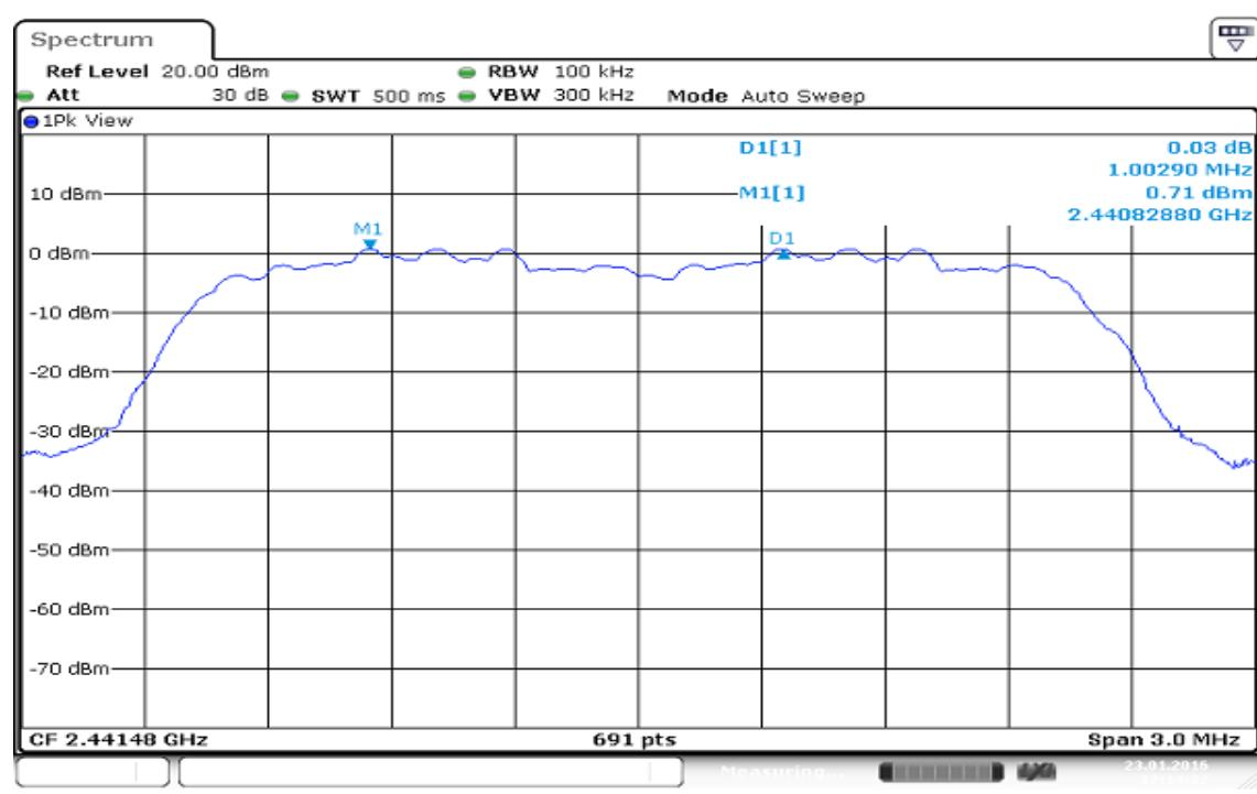
**Measurement of Channel Separation / (CH High)**
