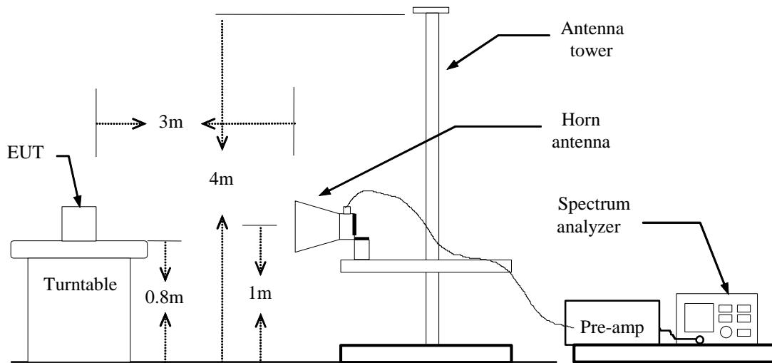
**Substituted Method Test Set-up**
