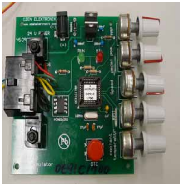
Figure 4.2 J1939 truck simulator
