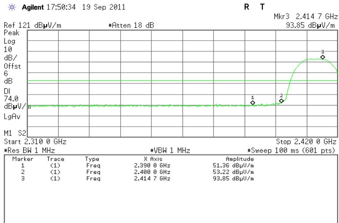
**Detector mode: Average****Polarity: Horizontal**
