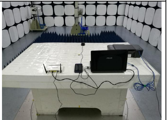
Radiated Emissions Test Setup Above 1GHz
