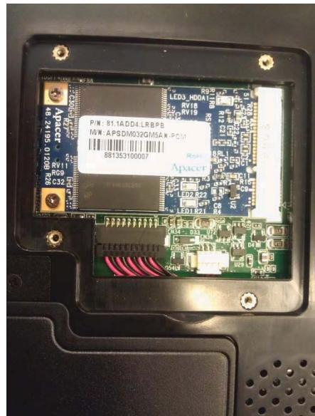
2. Unscrew and remove SSD from the slot.
