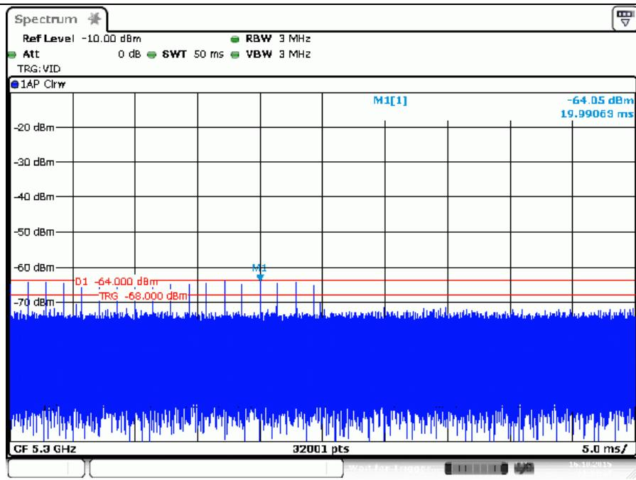
**Radar test signal type 1 / 5500MHz**
