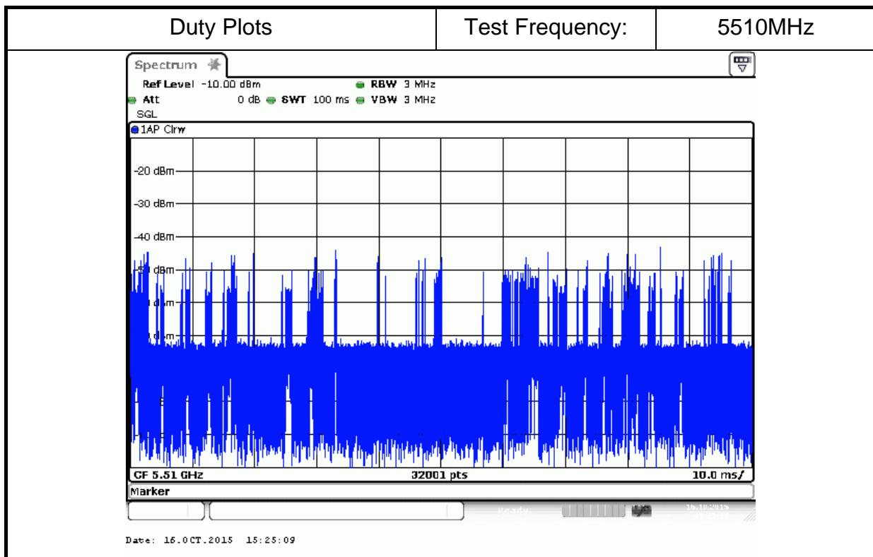
**Test Result of Channel Shutdown Time Plots**
