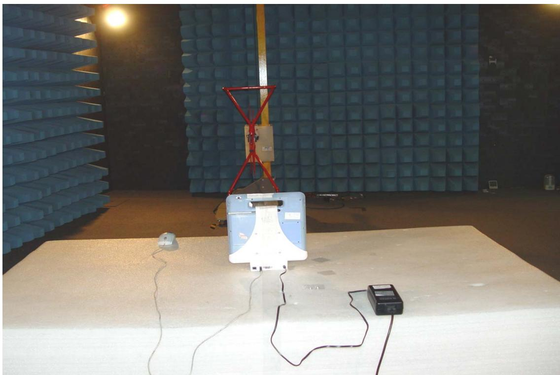
**POWERLINE CONDUCTED EMISSIONS SETUP PHOTOS**
