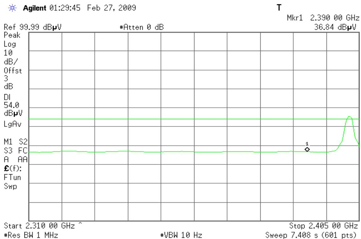
**Band Edges (CH High)****Detector mode: Peak****Polarity: Vertical**
