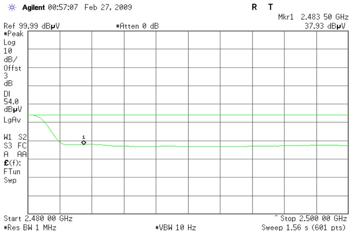
**For 8DPSK / DH5****Band Edges (CH Low)****Detector mode: Peak****Polarity: Vertical**
