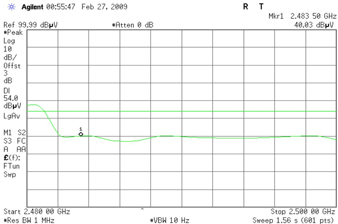
**Detector mode: Peak****Polarity: Horizontal**
