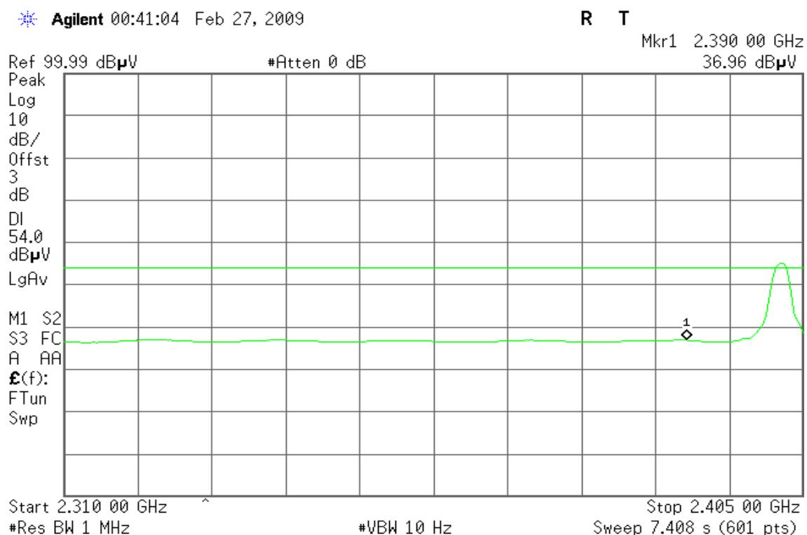
**Band Edges (CH High)****Detector mode: Peak****Polarity: Vertical**
