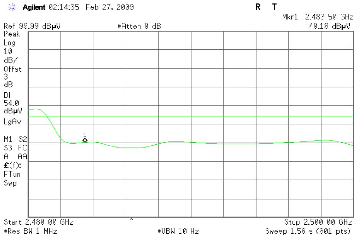
**Detector mode: Peak****Polarity: Horizontal**
