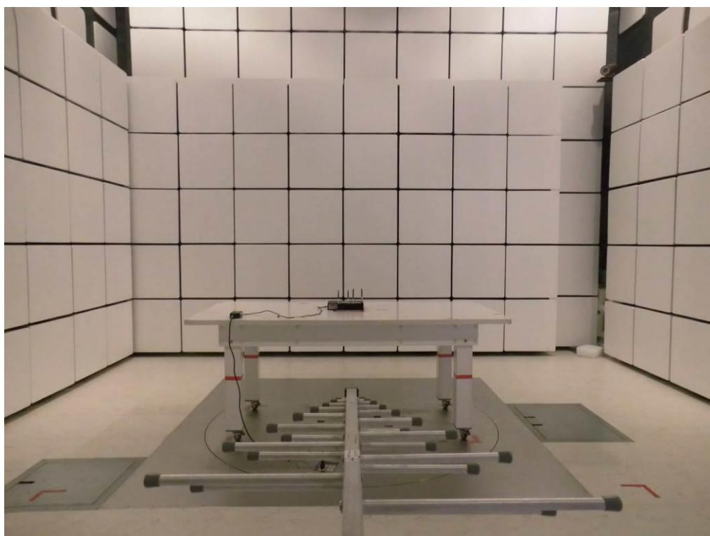
**Transmitter Radiated Emissions Test Photos****Above 1000 MHz**
