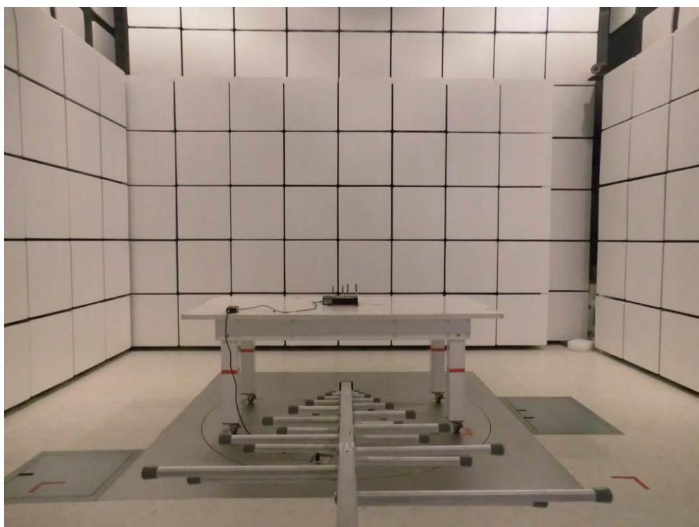
**Transmitter Radiated Emissions Test Photos****Above 1000 MHz**
