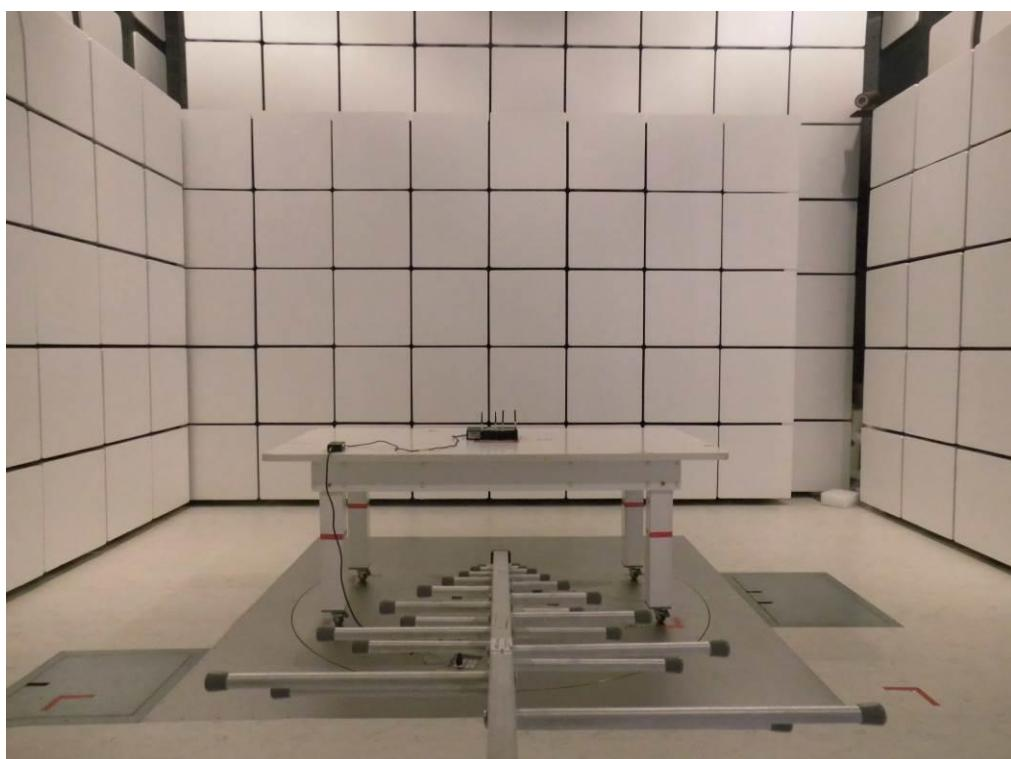
**Transmitter Radiated Emissions Test Photos****Above 1000 MHz**
