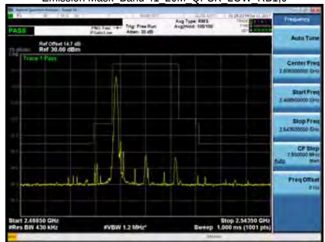
Emission Mask Band 41 20M QPSK LOW RB1,0
