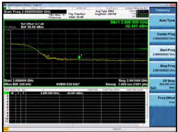
Band Edge_Band41 15MHz_QPSK 75 0_HighCH41165-2647.5
