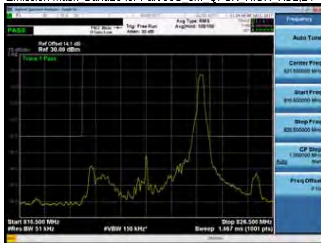
Emission Mask Band26 for Part 90S 5M QPSK HIGH RB1,24
