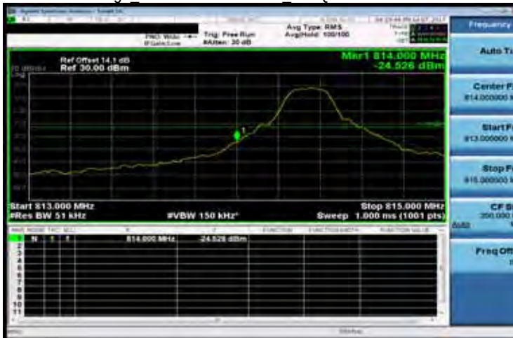
Band Edge Band 26 for Part 90S 5M-QPSK-1 0-LOW
