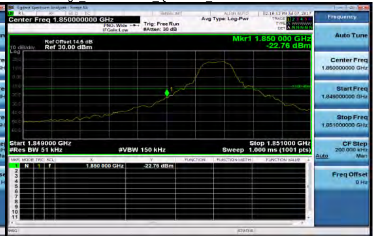
Band Edge Band25 5MHz QPSK 1 0 LowCH26065-1852.5
