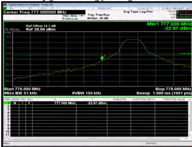
Band Edge Band13 5MHz QPSK 1 0 LowCH23205-779.5
