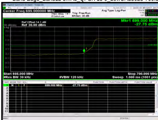
Band Edge_Band12 3MHz_QPSK 15 0_LowCH23025-700.5
