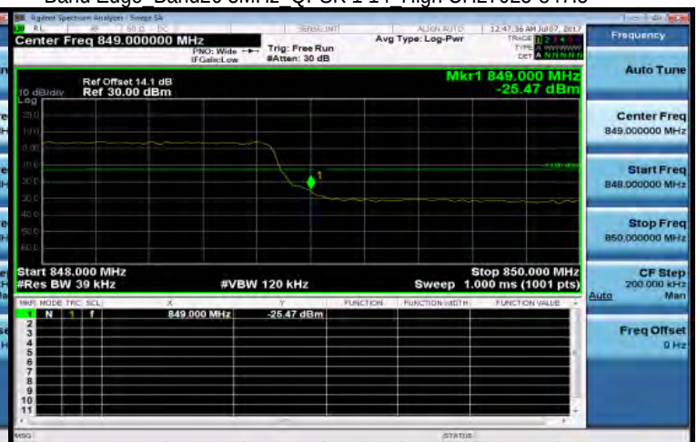
Band Edge_Band26 3MHz_QPSK 1 14_High CH27025-847.5
