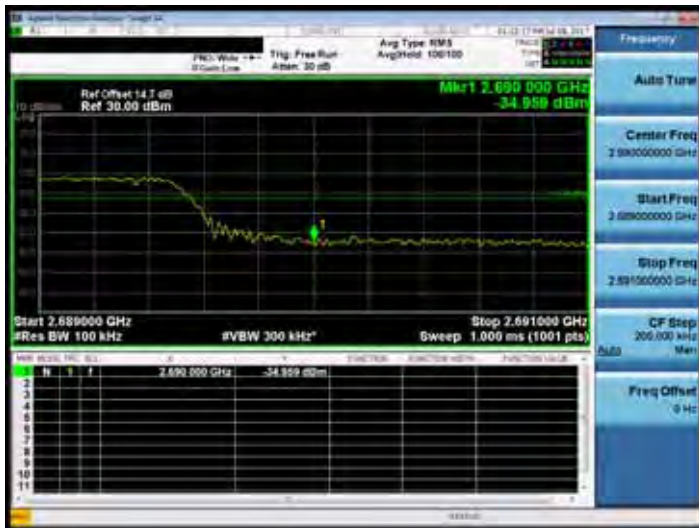
Band Edge_Band41 15MHz_QPSK 1 0_LowCH40215-2552.5
