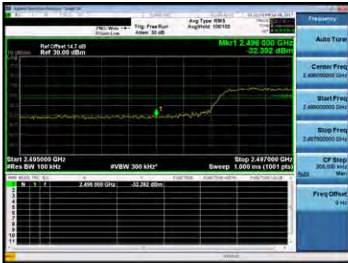
Band Edge_Band41 10MHz_QPSK 50 0_HighCH41190-2650
