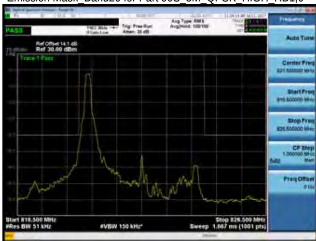
Emission Mask Band26 for Part 90S 5M QPSK HIGH RB1,0
