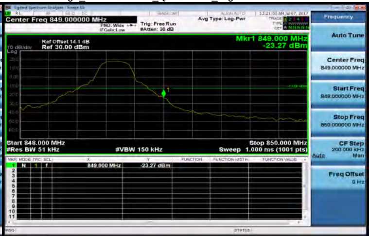
Band Edge Band26 5MHz QPSK 1 24 High CH27015-846.5
