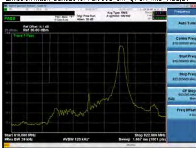
Emission Mask Band26 for Part 90S 3M QPSK MID RB1,14
