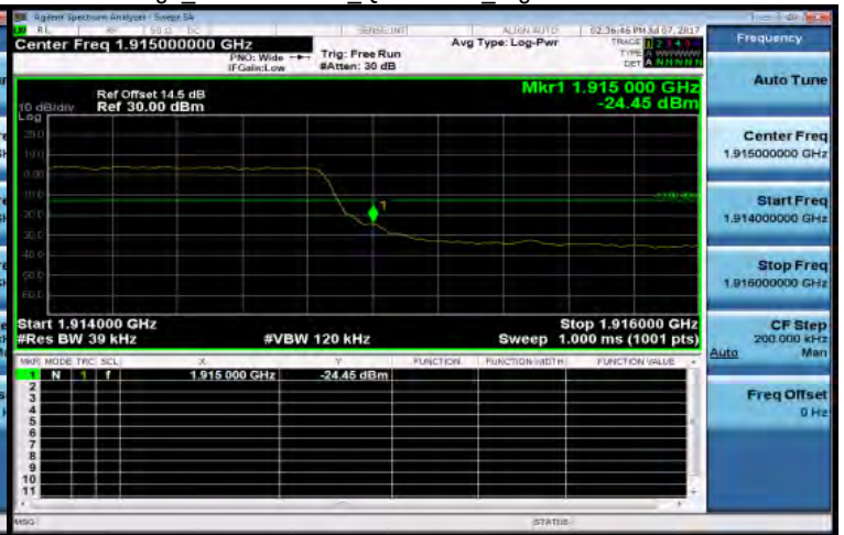
Band Edge Band25 3MHz QPSK 15 0 HighCH26675-1913.5
