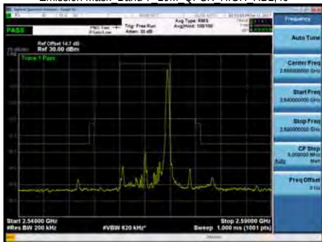
Emission Mask Band 7 10M QPSK HIGH RB1,49
