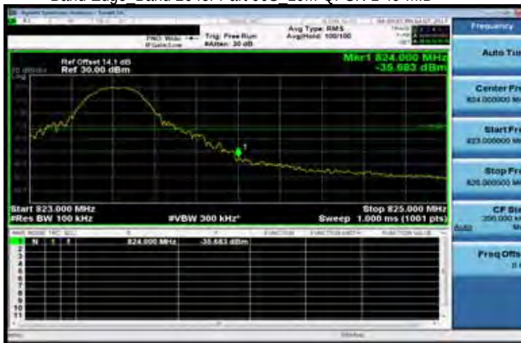
Band Edge Band 26 for Part 90S 10M-QPSK-1 49-MID
