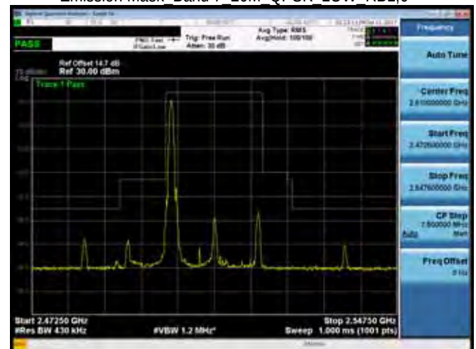
Emission Mask Band 7 20M QPSK LOW RB1,0
