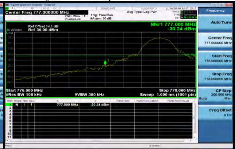
Band Edge Band13 10MHz QPSK 1 0 LowCH23230-782
