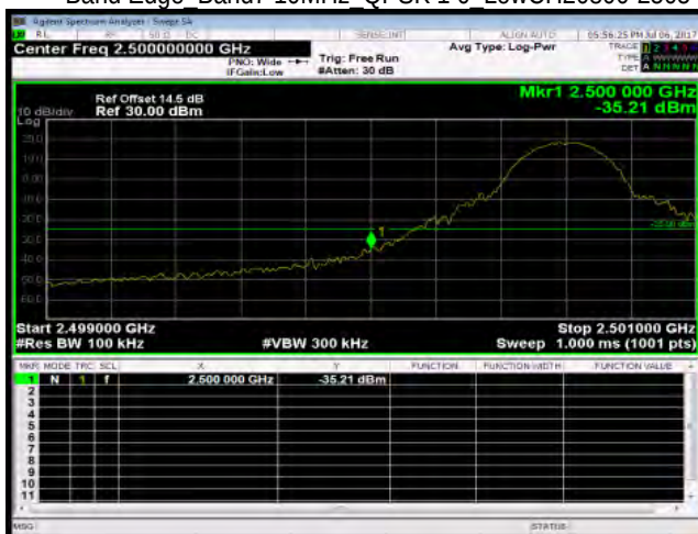
Band Edge Band7 10MHz QPSK 1 0 LowCH20800-2505
