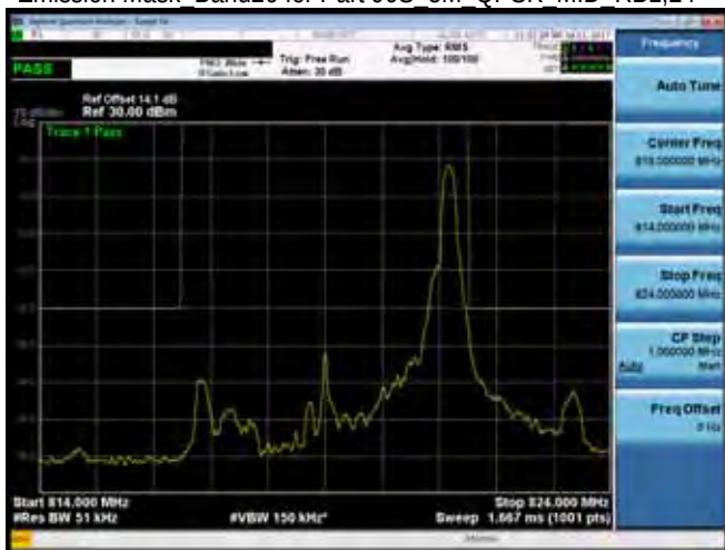
Emission Mask Band26 for Part 90S 5M QPSK MID RB1,24
