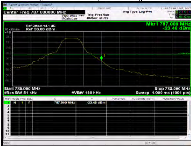
Band Edge Band13 5MHz QPSK 1 24 HighCH23255-784.5
