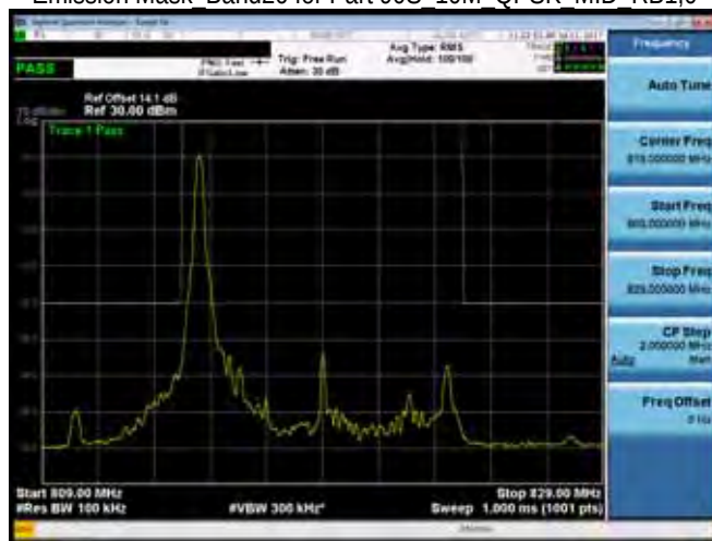
Emission Mask Band26 for Part 90S 10M QPSK MID RB1,0
