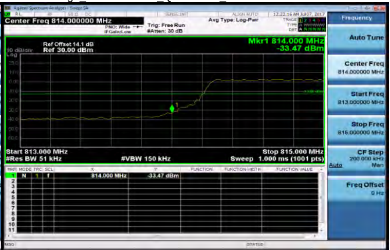
Band Edge Band26 5MHz QPSK 25 0 Low CH26815-826.5
