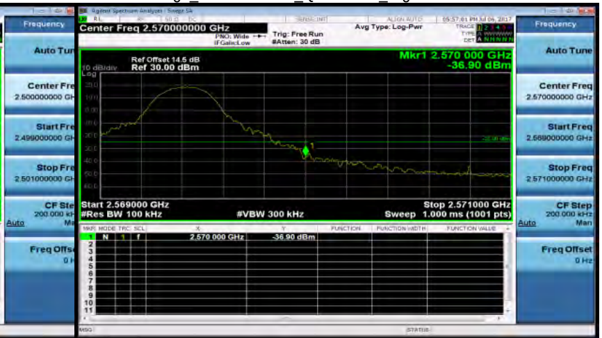
Band Edge Band7 10MHz QPSK 1 49 HighCH21400-2565
