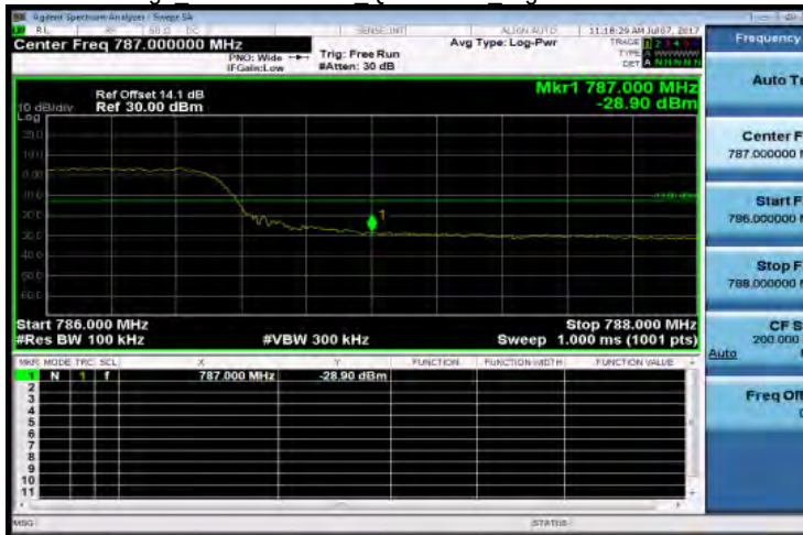
Band Edge_Band13 10MHz_QPSK 50 0_HighCH23230-782
