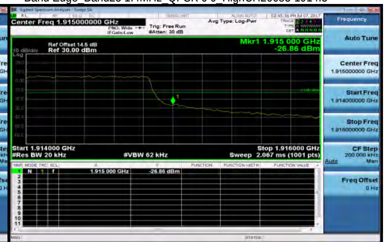
Band Edge_Band25 1.4MHz_QPSK 6 0_HighCH26683-1914.3
