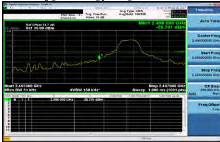
Band Edge Band41 5MHz QPSK 1 0 LowCH40165-2547.5
