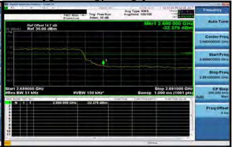
Band Edge Band41 5MHz QPSK 25 0 HighCH41215-2652.5
