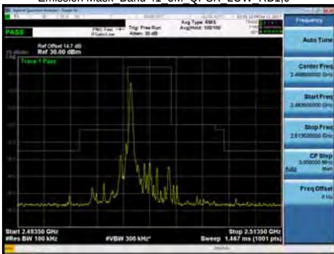
Emission Mask Band 41 5M QPSK LOW RB1,0
