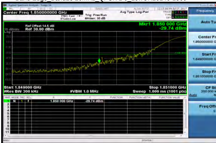
Band Edge Band25 20MHz QPSK 1 0 LowCH26140-1860
