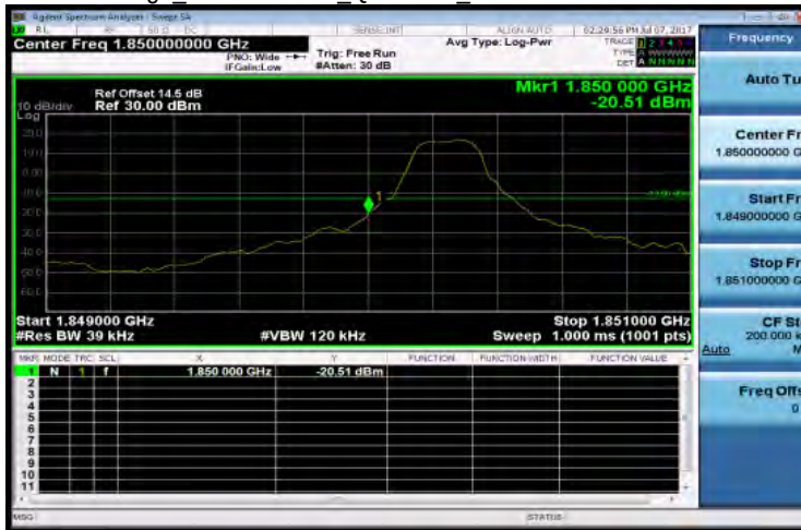
Band Edge Band25 3MHz QPSK 1 0 LowCH26055-1851.5
