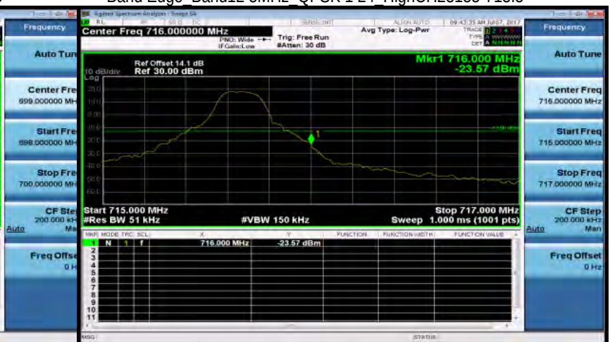
Band Edge_Band12 5MHz_QPSK 1 24_HighCH23155-713.5
