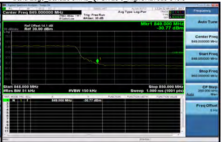
Band Edge Band26 5MHz QPSK 25 0 High CH27015-846.5
