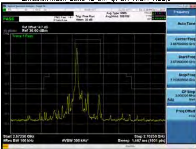
Emission Mask Band 41 5M QPSK HIGH RB1,0
