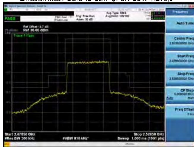
Emission Mask Band 41 15M QPSK MID RB1,0
