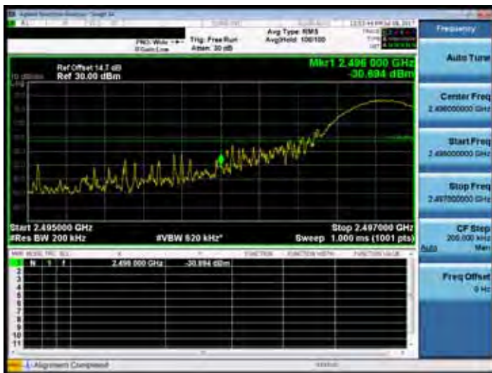
Band Edge_Band41 15MHz_QPSK 1 0_LowCH40215-2552.5
