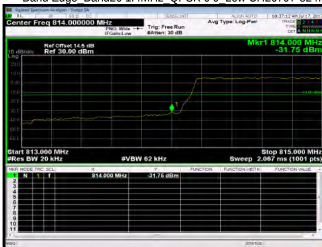
Band Edge_Band26 1.4MHz_QPSK 6 0_Low CH26797-824.7
