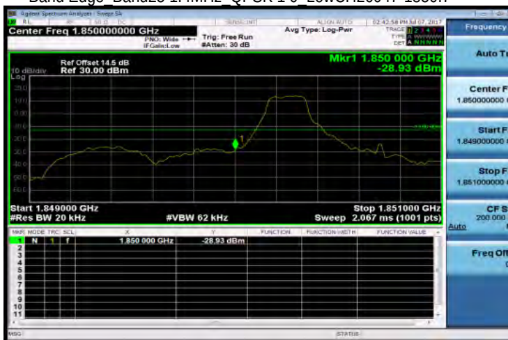
Band Edge_Band25 1.4MHz_QPSK 1 0_LowCH26047-1850.7
