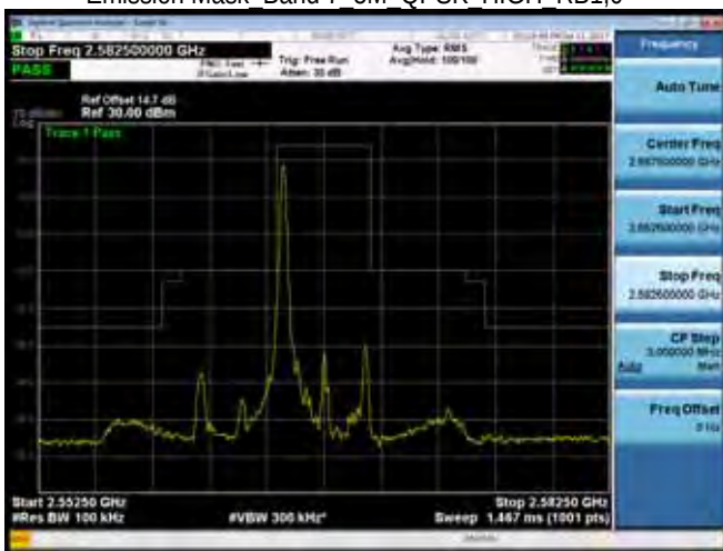
Emission Mask Band 7 5M QPSK HIGH RB1,0
