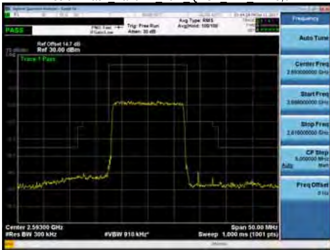
Emission Mask Band 41 15M QPSK HIGH RB1,0
