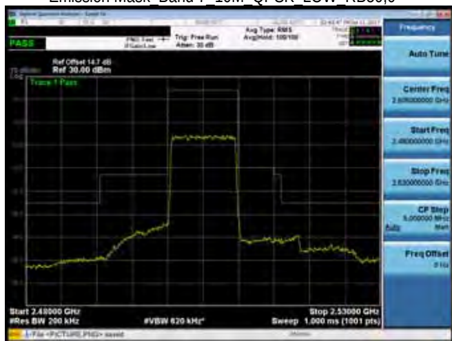
Emission Mask Band 7 10M QPSK MID RB1,0
