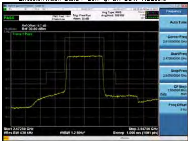
Emission Mask Band 7 20M QPSK MID RB1,0
