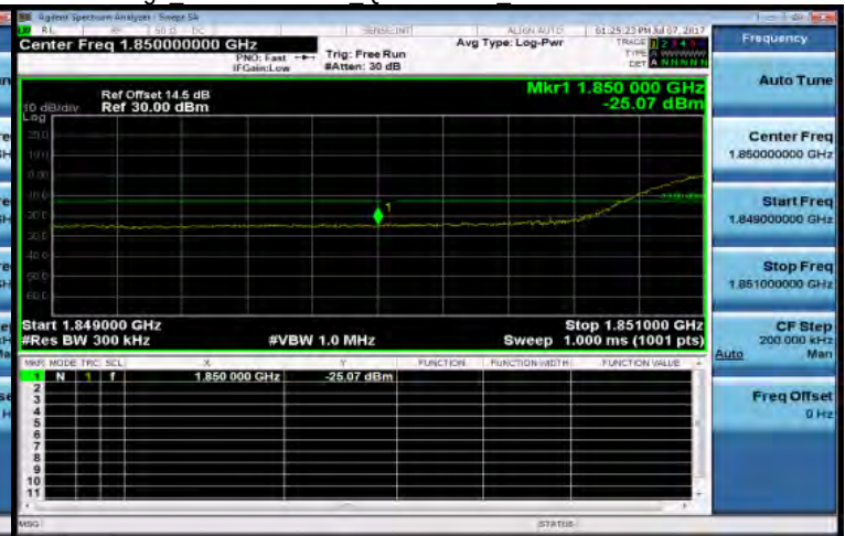
Band Edge Band25 20MHz QPSK 100 0 LowCH26140-1860
