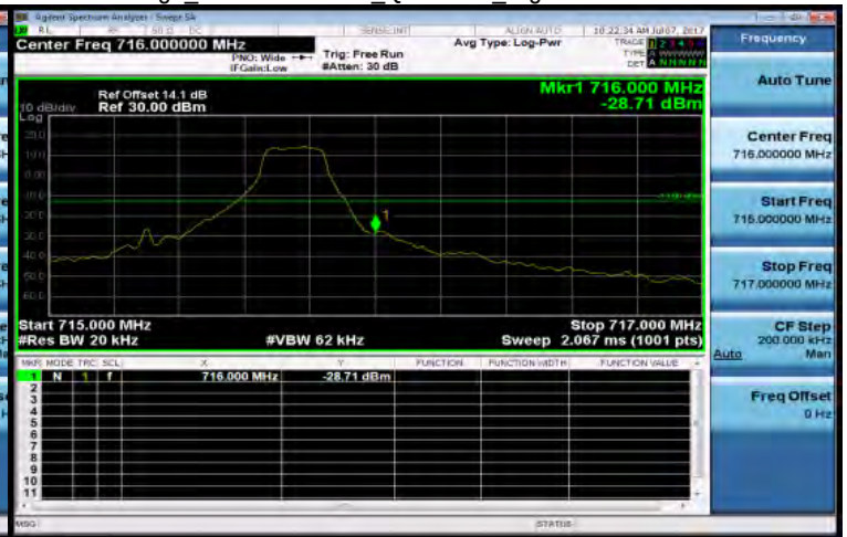
Band Edge_Band12 1.4MHz_QPSK 1 5_HighCH23173-715.3
