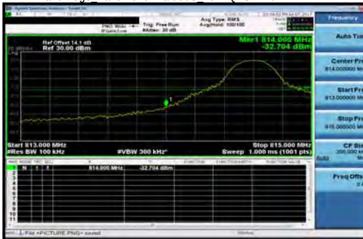
Band Edge Band 26 for Part 90S 10M-QPSK-1 0-MID
