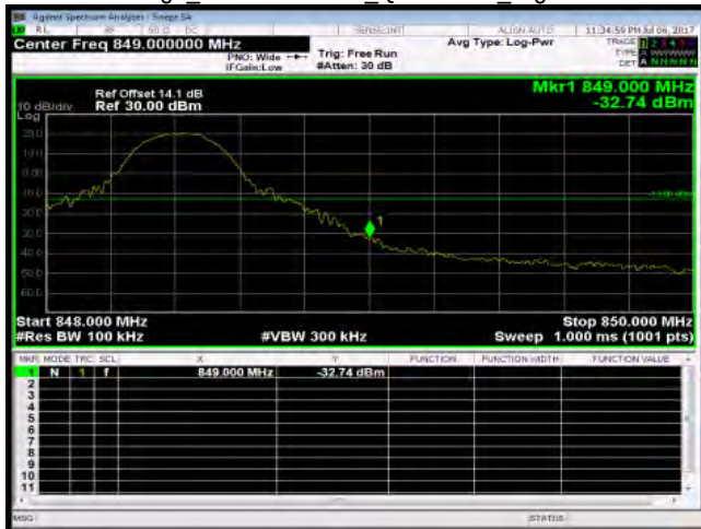
Band Edge_Band26 10MHz_QPSK 1 49_HighCH26990-844
