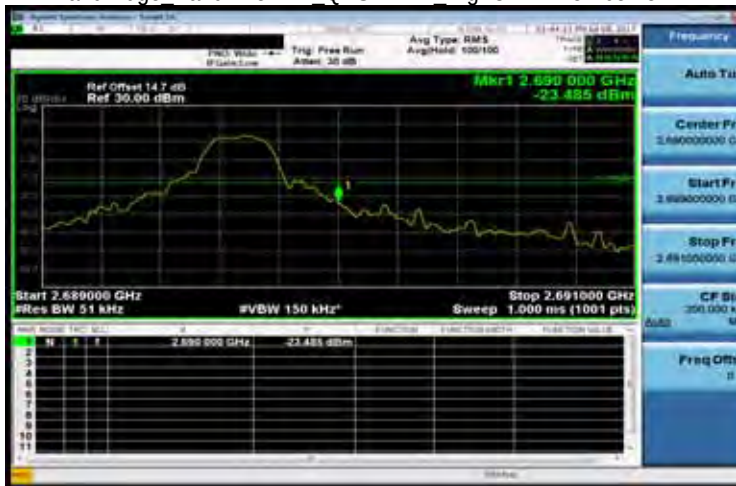
Band Edge Band41 5MHz QPSK 1 24 HighCH41215-2652.5
