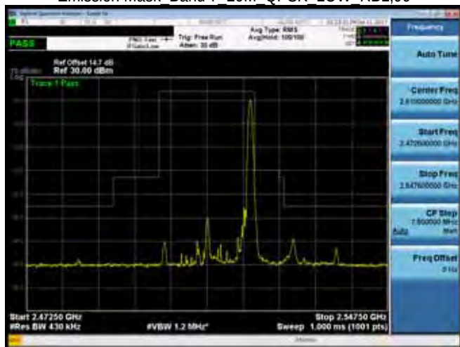
Emission Mask Band 7 20M QPSK LOW RB1,99
