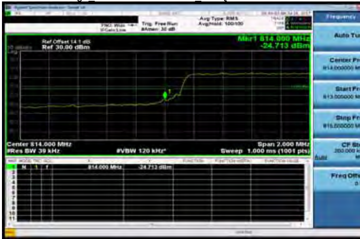
Band Edge Band 26 for Part 90S 3M-QPSK-15 0-LOW
