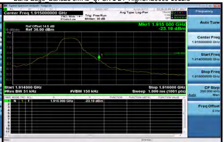
Band Edge Band25 5MHz QPSK 1 24 HighCH26665-1912.5
