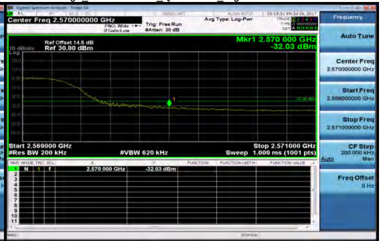
Band Edge Band7 15MHz QPSK 75 0 HighCH21375-2562.5
