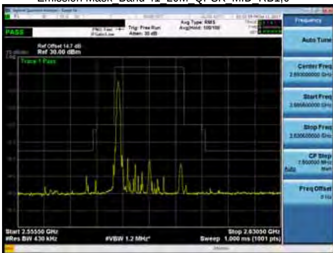
Emission Mask Band 41 20M QPSK MID RB1,0
