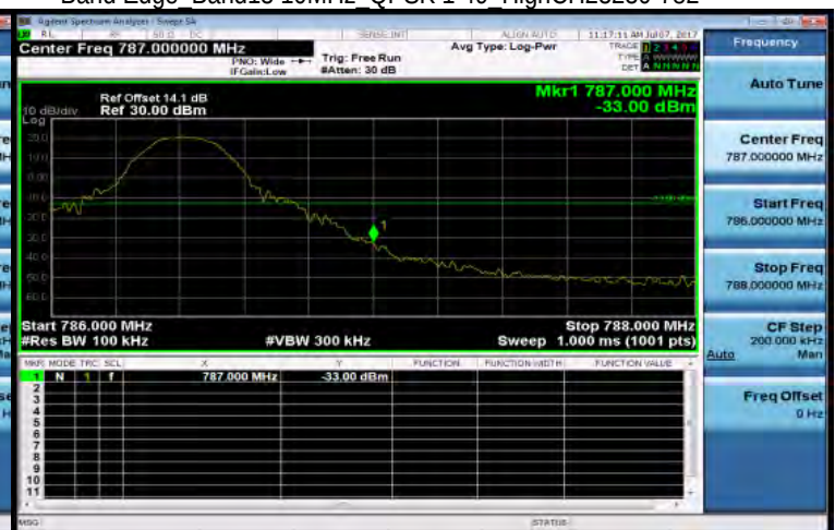
Band Edge Band13 10MHz QPSK 1 49 HighCH23230-782
