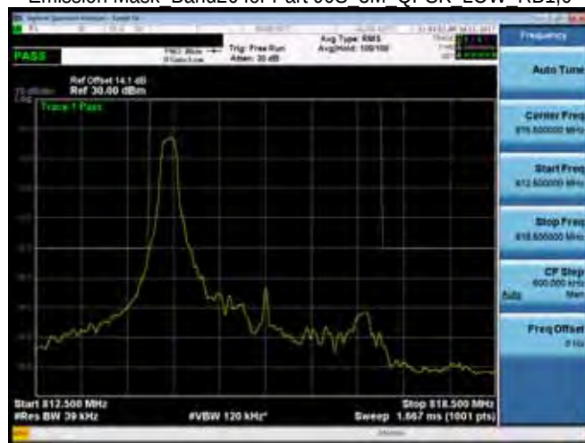
Emission Mask Band26 for Part 90S 3M QPSK LOW RB1,0
