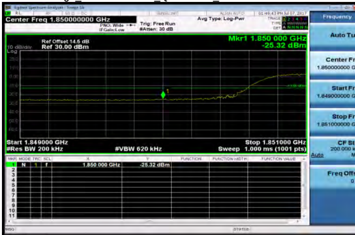
Band Edge Band25 15MHz QPSK 75 0 LowCH26115-1857.5
