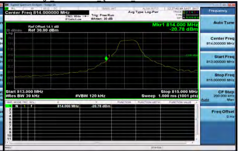
Band Edge_Band26 3MHz_QPSK 1 0_Low CH26805-825.5
