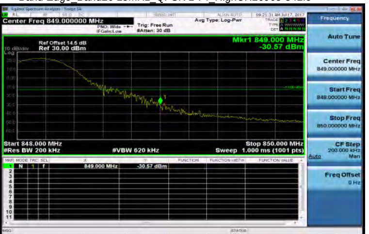
Band Edge_Band26 15MHz_QPSK 1 74_HighCH26965-841.5
