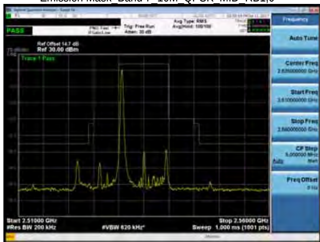
Emission Mask Band 7 10M QPSK MID RB1,0
