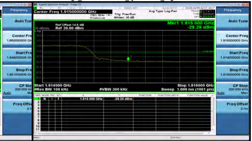
Band Edge_Band25 10MHz_QPSK 50 0_HighCH26640-1910
