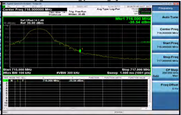
Band Edge Band12 10MHz QPSK 1 49 HighCH23130-711
