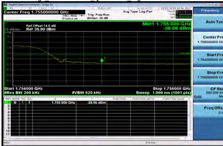
Band Edge Band4 15MHz QPSK 75 0 HighCH20325-1747.5
