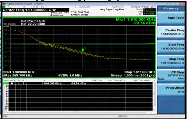
Band Edge Band2 20MHz QPSK 1 99 HighCH19100-1900
