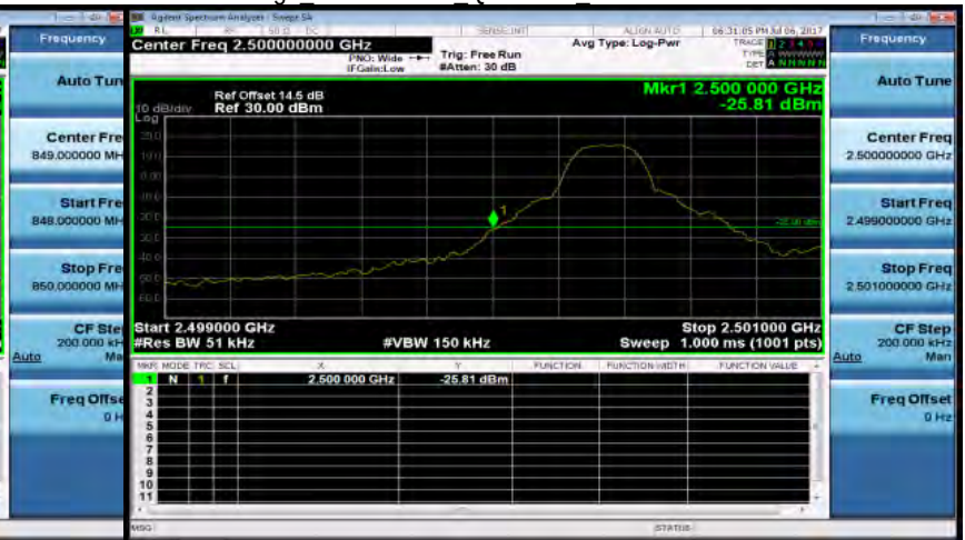
Band Edge Band7 5MHz QPSK 1 0 LowCH20775-2502.5
