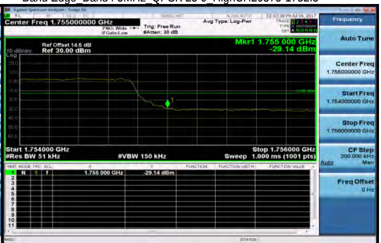
Band Edge Band4 5MHz QPSK 25 0 HighCH20375-1752.5
