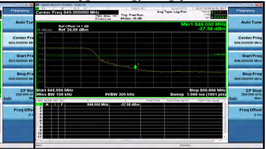
Band Edge Band5 10MHz QPSK 50 0 HighCH20600-844
