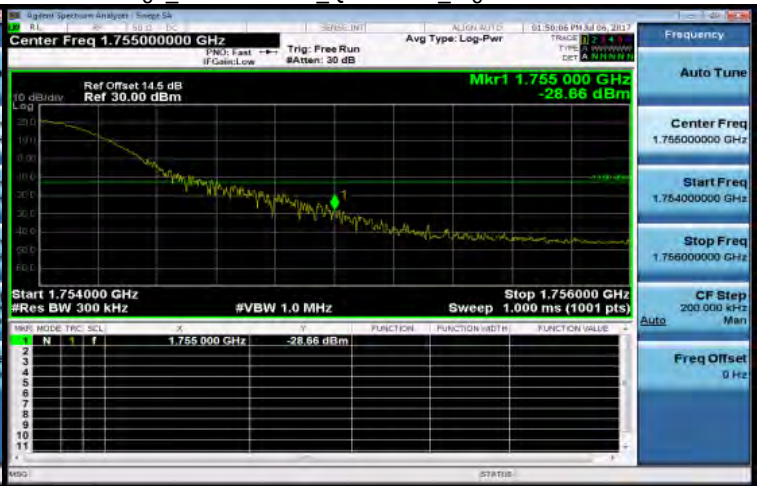
Band Edge Band4 20MHz QPSK 1 99 HighCH20300-1745
