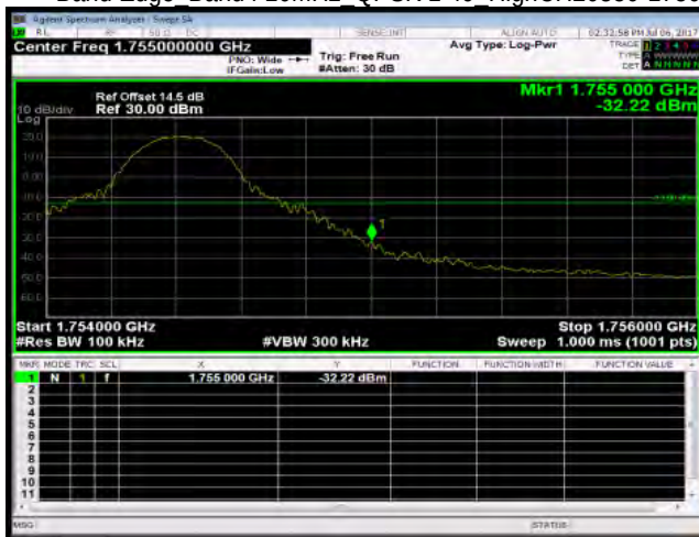
Band Edge Band4 10MHz QPSK 1 49_HighCH20350-1750
