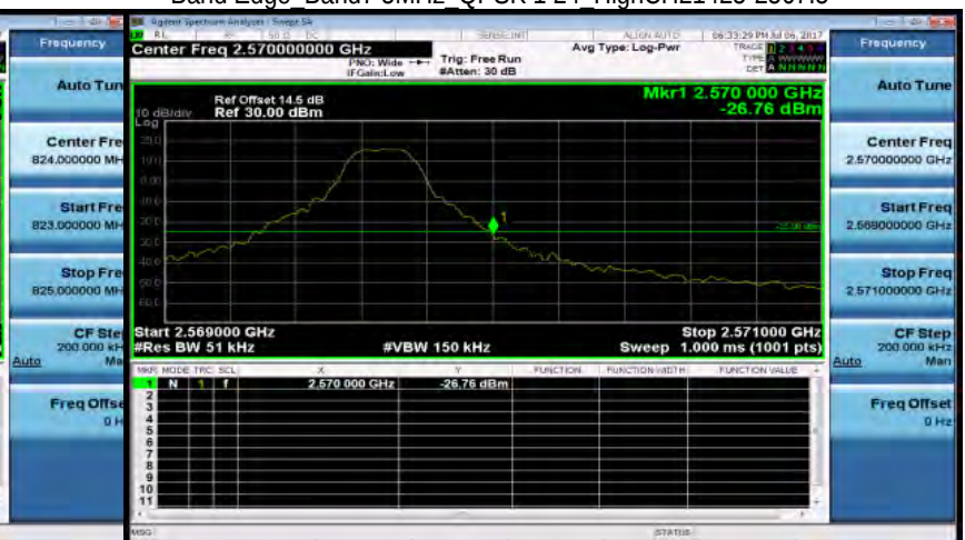
Band Edge Band7 5MHz QPSK 1 24 HighCH21425-2567.5
