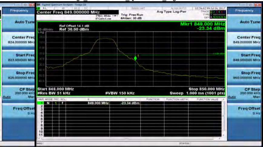
Band Edge_Band5 5MHz_QPSK 1 24_HighCH20625-846.5
