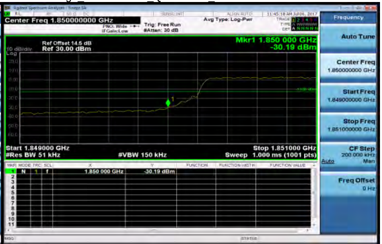
Band Edge Band2 5MHz QPSK 25 0 LowCH18625-1852.5
