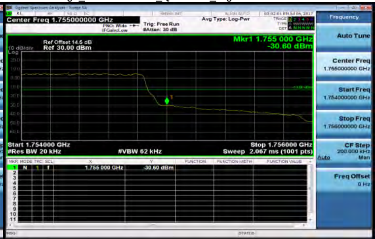
Band Edge_Band4 1.4MHz QPSK 6 0 HighCH20393-1754.3
