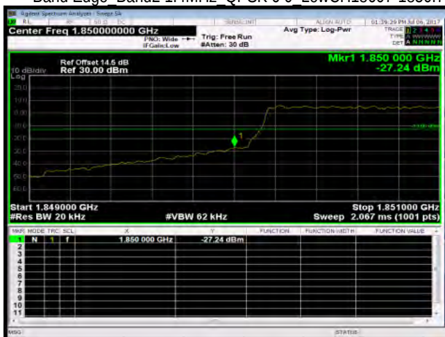
Band Edge_Band2 1.4MHz QPSK 6 0 LowCH18607-1850.7
