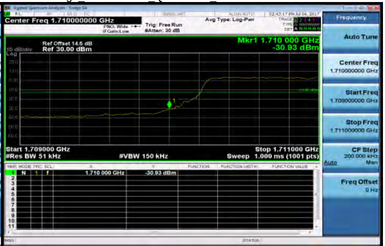
Band Edge Band4 5MHz QPSK 25 0 LowCH19975-1712.5
