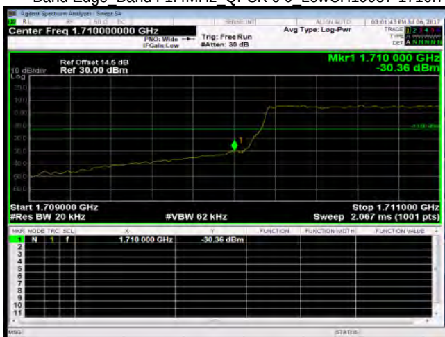
Band Edge_Band4 1.4MHz QPSK 6 0 LowCH19957-1710.7
