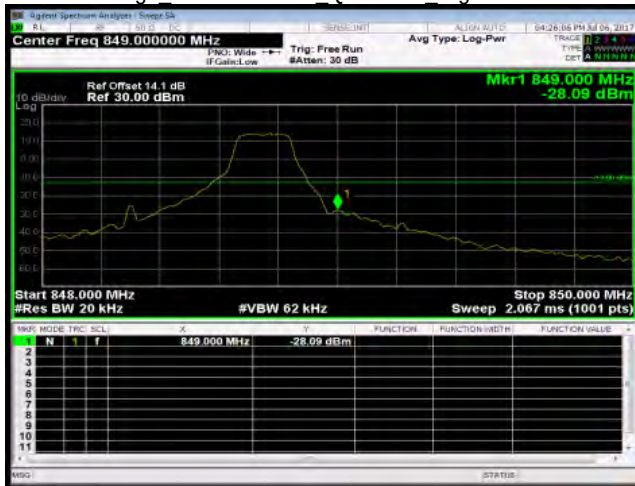
Band Edge_Band5 1.4MHz_QPSK 1 5_HighCH20643-848.3
