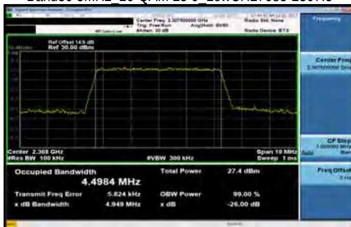
Band30 5MHz_16-QAM 25 0_LowCH27685-2307.5
