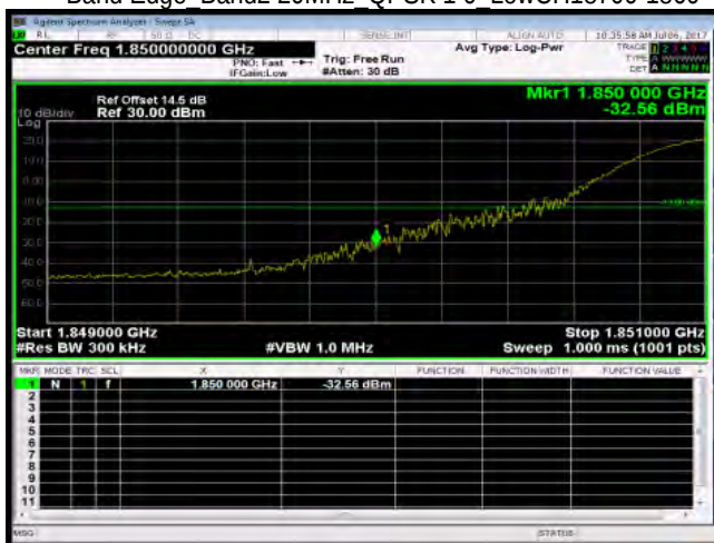
Band Edge Band2 20MHz QPSK 1 0 LowCH18700-1860
