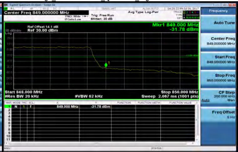
Band Edge_Band5 1.4MHz_QPSK 6 0_HighCH20643-848.3
