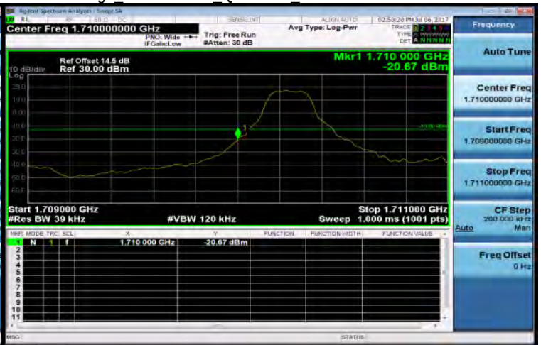
Band Edge_Band4 3MHz QPSK 1 0 LowCH19965-1711.5
