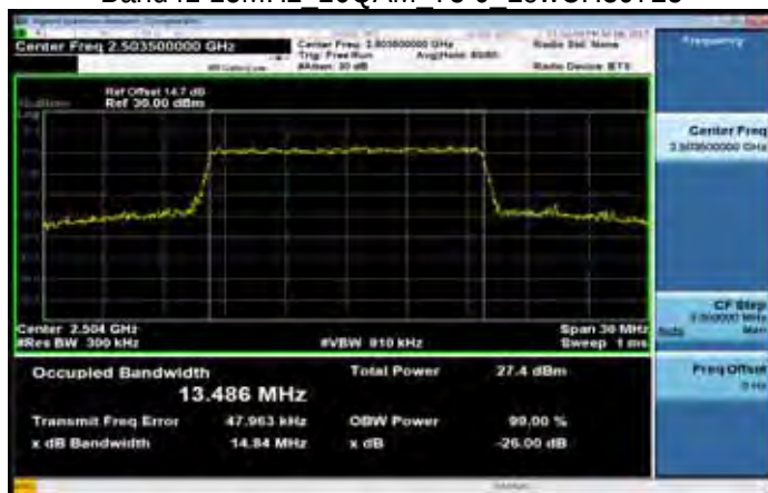
Band41 15MHz 16QAM 75 0 LowCH39725
