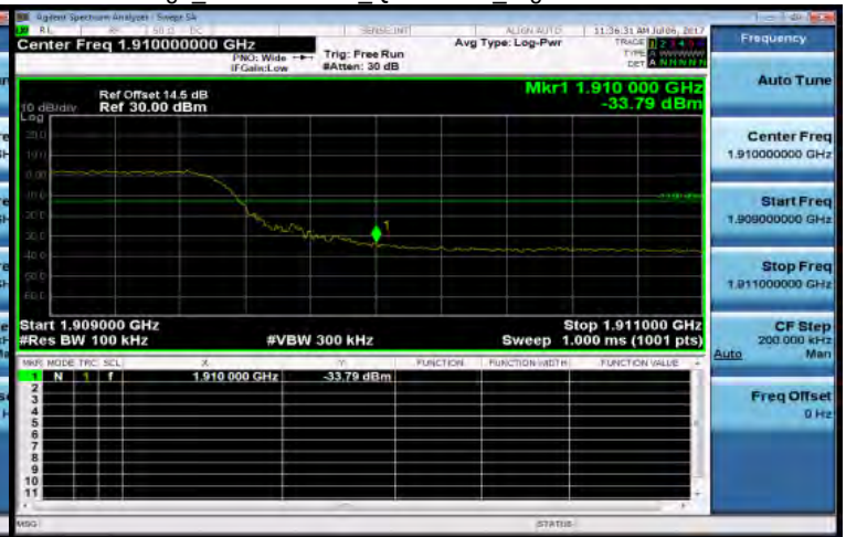
Band Edge_Band2 10MHz_QPSK 50 0_HighCH19150-1905
