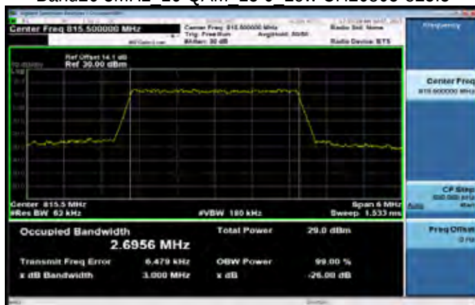
Band26 3MHz_16-QAM_15_0_Low CH26805-825.5
