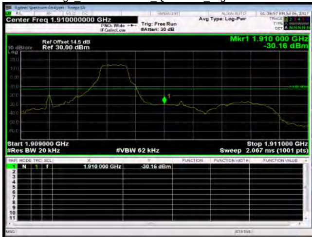
Band Edge_Band2 1.4MHz QPSK 1 5 HighCH19193-1909.3
