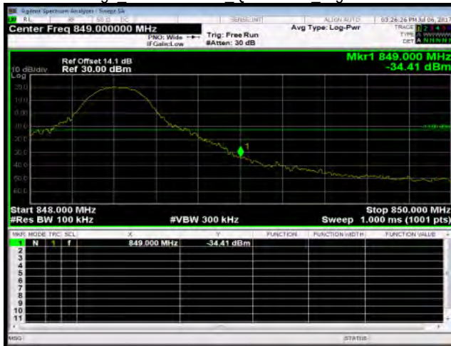
Band Edge Band5 10MHz QPSK 1 49 HighCH20600-844
