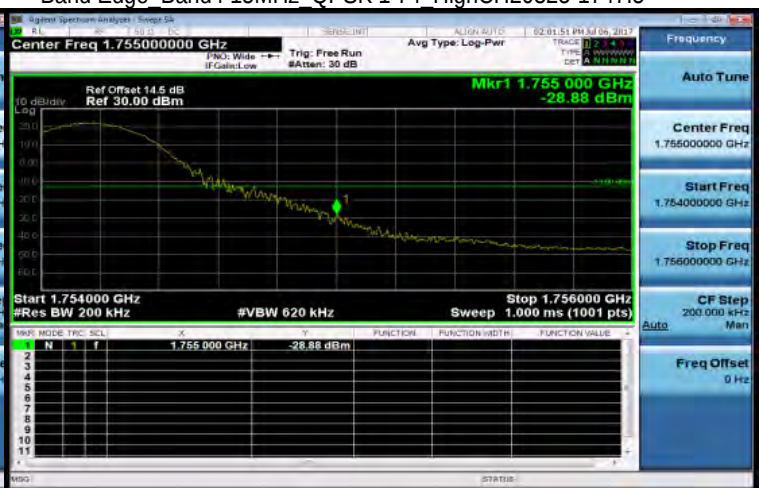
Band Edge Band4 15MHz QPSK 1 74_HighCH20325-1747.5
