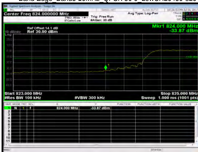
Band Edge Band5 10MHz QPSK 50 0 LowCH20450-829
