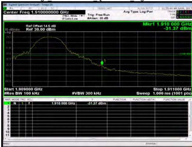
Band Edge_Band2 10MHz_QPSK 1 49_HighCH19150-1905
