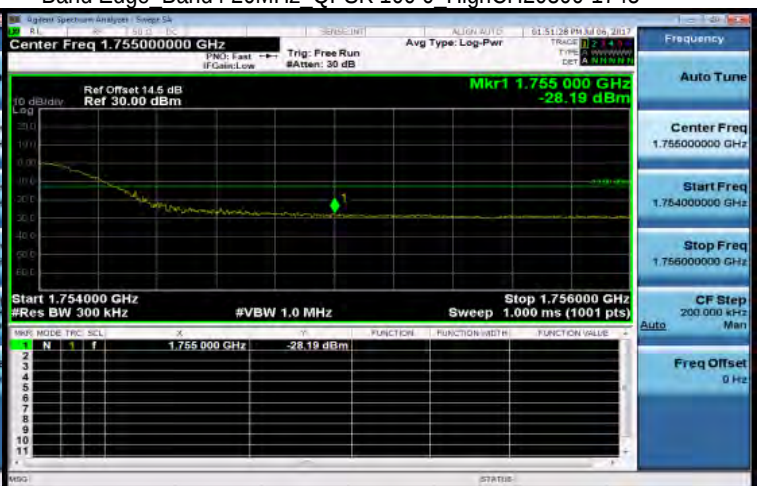
Band Edge Band4 20MHz QPSK 100 0 HighCH20300-1745
