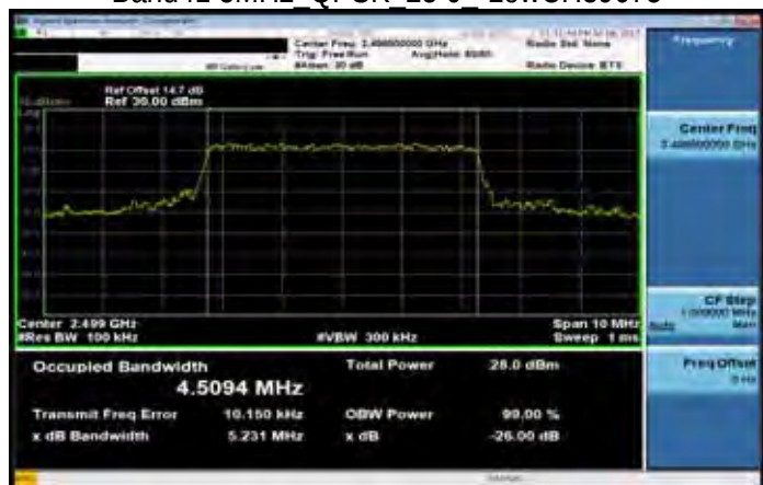
Band41 5MHz QPSK 25 0 LowCH39675
