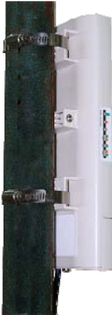
Figure 8 Pole Mounting – Step 2
