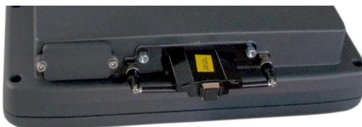
Fig. 7.9: WLAN, WWAN LTE 4G antenna opened
