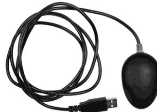
Fig. 6.5: External GPS receiver (optional)
