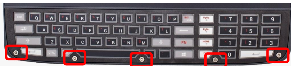
Fig. 16.1: Integrated keyboard: Unscrew the mounting screws
