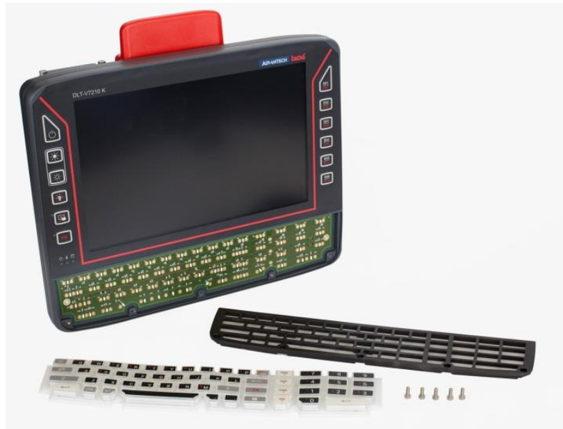
Fig. 16.2: Integrated keyboard: Keyboard components
