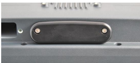
Fig. 7.3: DLT-V72 with a sealing plate (no radio antenna)
