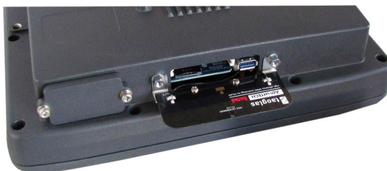
Fig. 7.6: WLAN antenna IEEE 802.11 a/b/g/n/ac opened
