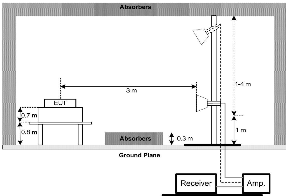
**(C) Radiated emissions below 30MHz**
