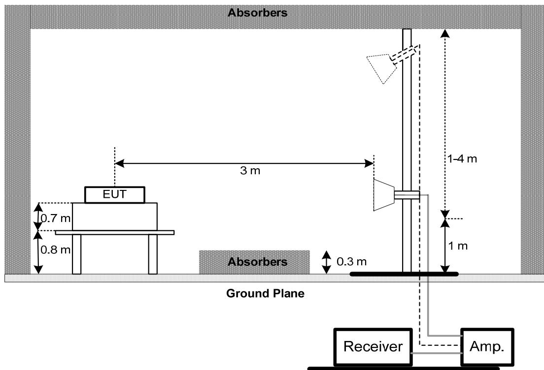
(C) For Radiated Emissions Below 30MHz
