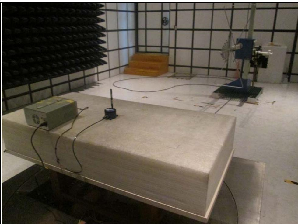
RADIATED EMISSION TEST (Mode A)
