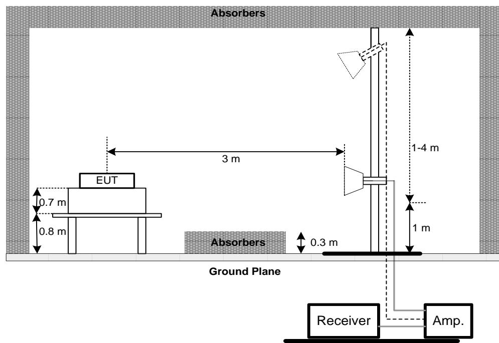
(C) For radiated emissions below 30MHz
