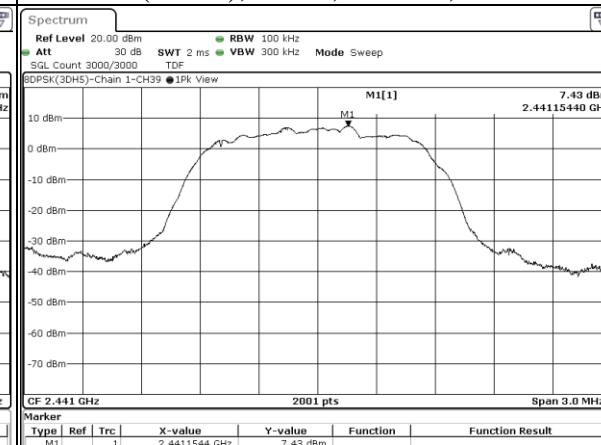
**8DPSK(3DH5), CH39, Chain 1, Conducted Emission**
