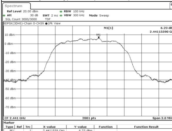
**8DPSK(3DH5), CH39, Chain 0, Conducted Emission**
