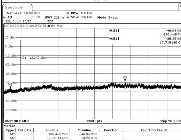
**8DPSK(3DH5), CH78, Chain 1, Conducted Emission**
