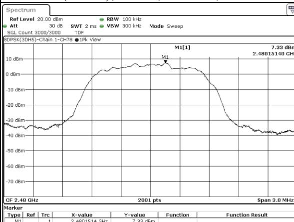
**8DPSK(3DH5), CH78, Chain 0, Conducted Emission**
