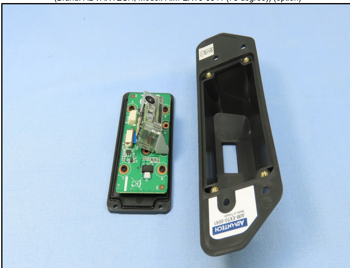
Extension Modules- Barcode scanner (70° ) (Brand: ADVANTECH, Model: AIM-EXT0-0041 (70 degree)) (option)
