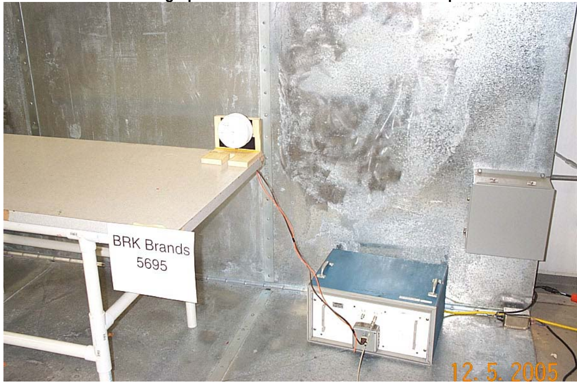
Photograph of Conducted Emissions Test Setup
