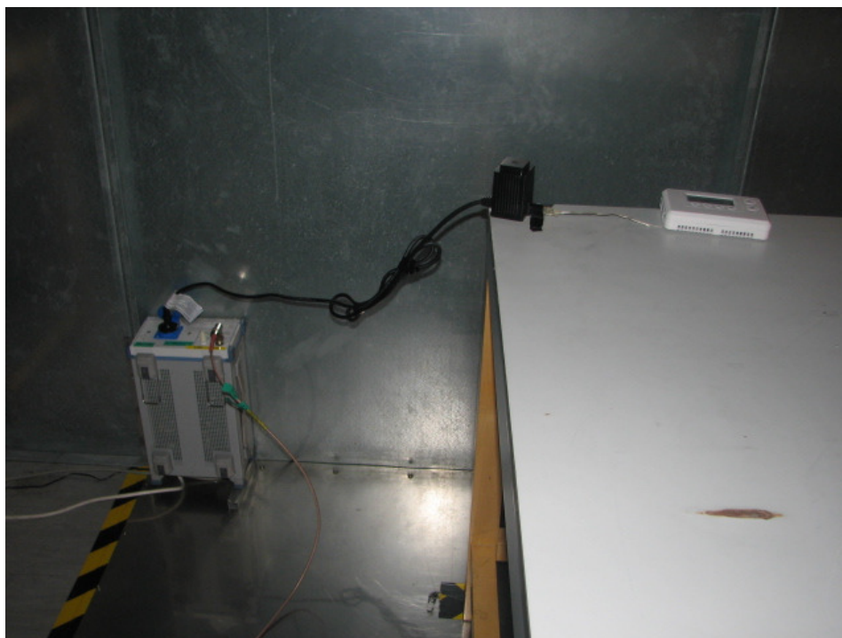
Set-up for Conducted Emission
