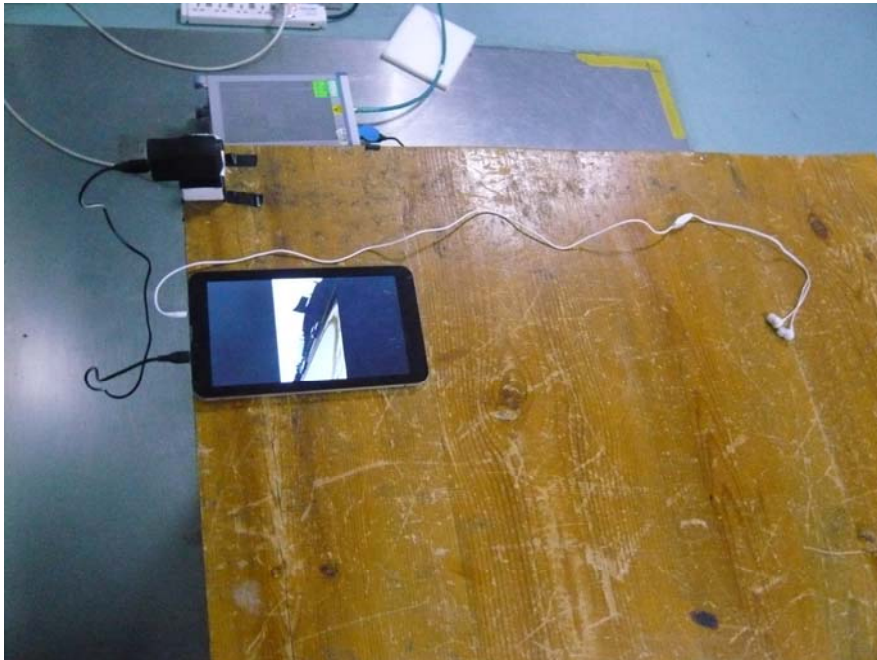
Conducted Emissions - Side View (Charging&Playing)
