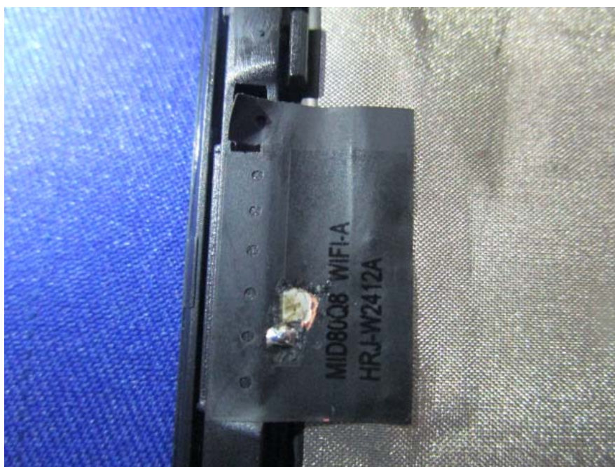
EUT –Wifi &BT Antenna View
