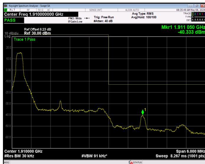
Band2 QPSK BW=3MHz Channel=19185 RB Size=15 Position=#0
