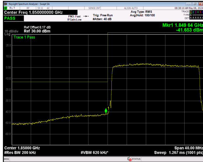
Band2 16QAM BW=20MHz Channel=19100 RB Size=1 Position=#0
