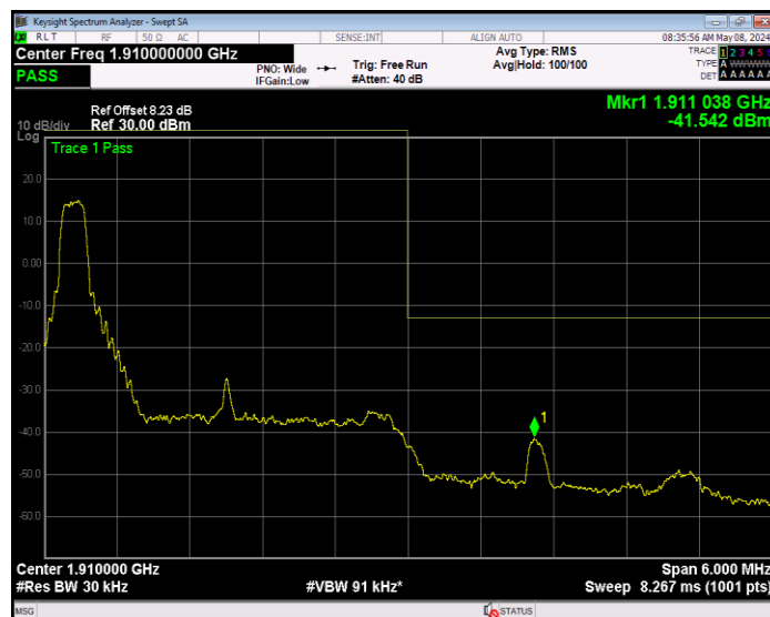
Band2 16QAM BW=3MHz Channel=19185 RB Size=15 Position=#0
