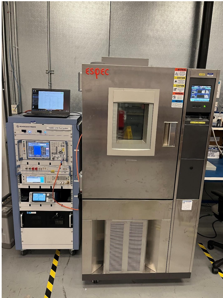
Conducted Antenna Port Measurements (external to environmental chamber)
