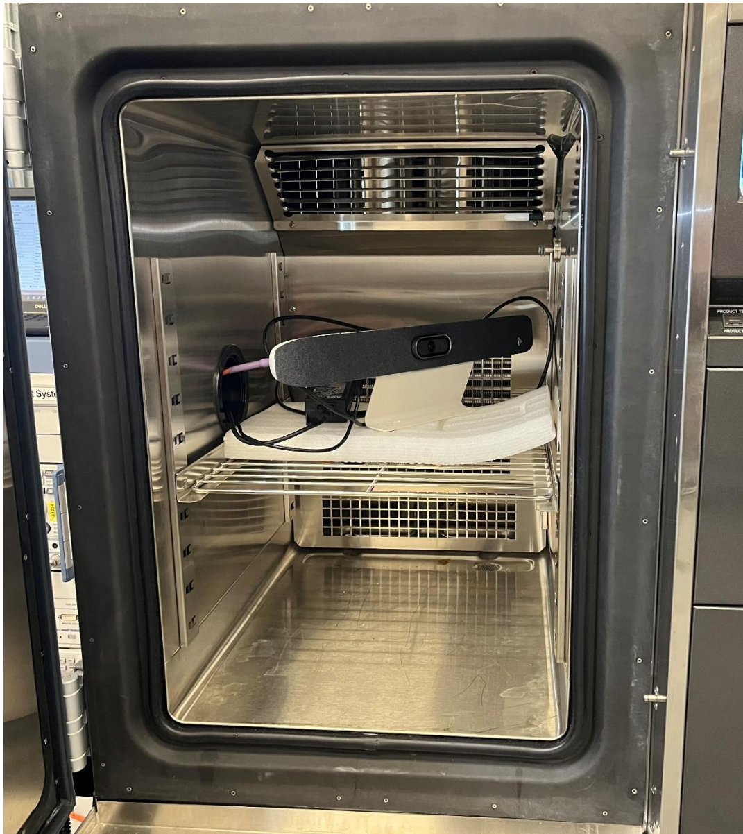
Conducted Antenna Port Measurements (internal to environmental chamber)
